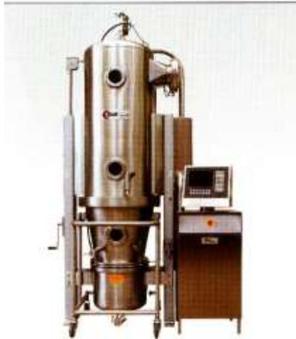
Machine capacities range from 125 to 1275 litres
