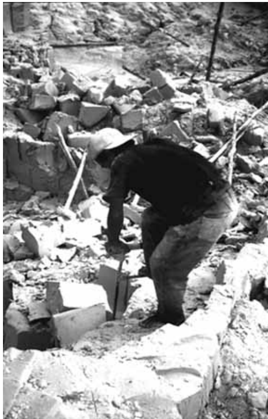
Figure 2: Ball Clay being mined with a tubal in Kalimantan Island, Indonesia.
