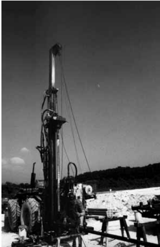
Figure 11: A Geological Exploration rig drilling for Ball Clay in Devon.
