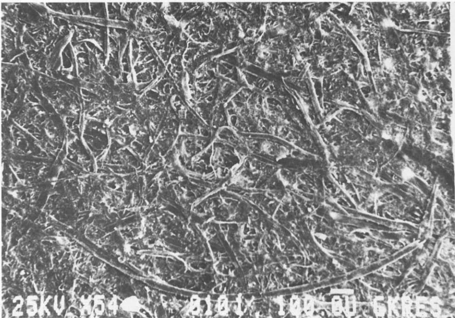
Fig. 3. Scanning electron micrograph of uncoated paper (after Bundy and Harrison, 1986).
