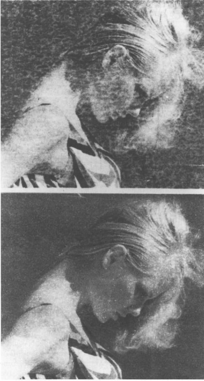
Fig. 5. Rotogravure signatures show (a) print mottle with calcined clay and (b) missing dots with Fine No. 1 product.
