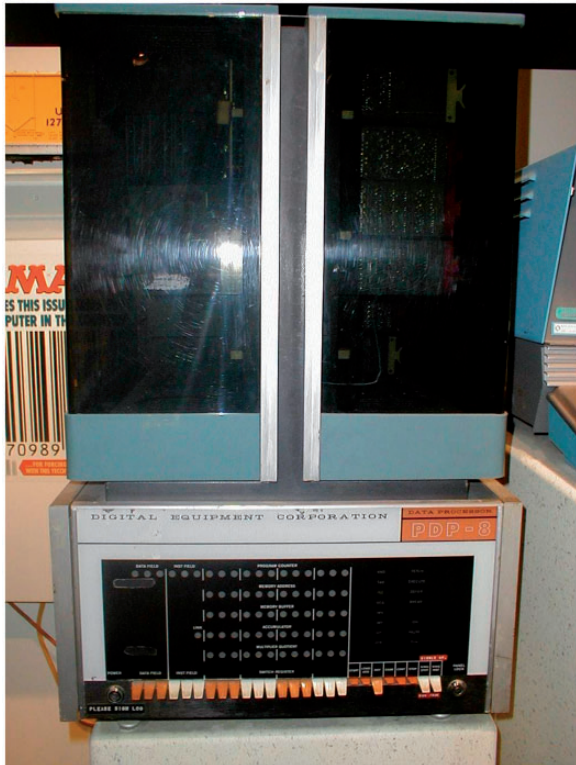
Illustration 1. The DEC PDP-8 Minicomputer, manufactured in 1965. The main processing module (pictured here) weighed 180 pounds and was sold at the introductory price of $18 500 (~$140 000 in 2018 dollars). Image: Wikimedia Commons//CCO.
