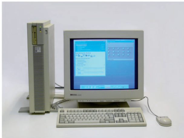
Illustration 3. An HP-9000 desktop workstation running the Unix-based system HP-UX. Image: Thomas Schanz//CC-BY-SA 3.0.
