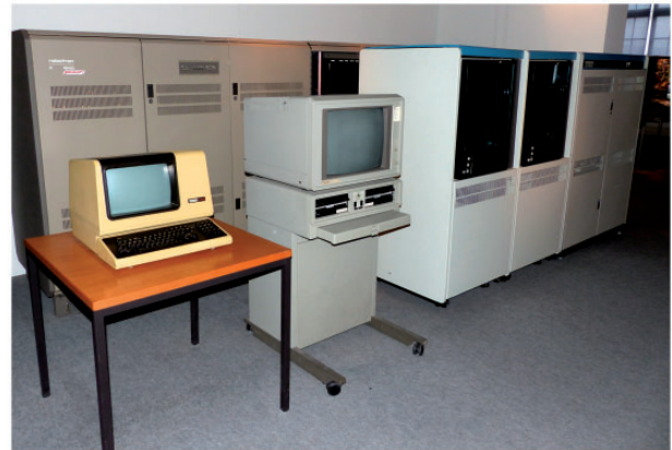
Illustration 2. The DEC VAX-11/780 Minicomputer. From right to left: The computer module, two tape storage units, a monitor and a terminal. The GCG software package was initially designed to run on this computer. Image: Wikimedia Commons//CCO.
