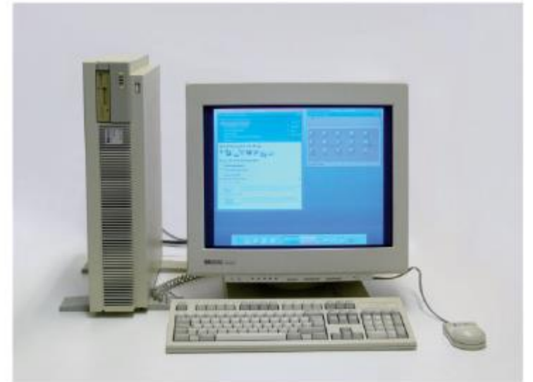
Illustration 3. An HP-9000 desktop workstation running the Unix-based system HP-UX. Image: Thomas Schanz//CC-BY-SA 3.0.
