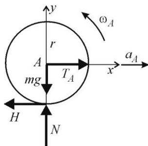
$$\begin{aligned} \text{TR: } ma_A \vec{i} &= (T_A - H) \vec{i} + (N - mg) \vec{j} \Rightarrow \\ \Rightarrow \begin{cases} ma_A = T_A - H \\ N = mg \end{cases} & \quad (1) \end{aligned}$$
