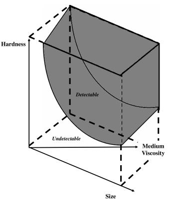
**Figure 9** Particle detectability as a function of hardness, size, and suspension medium viscosity.
