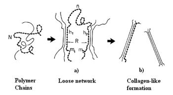
**Figure 8** Schematic of gelatin gelation. Two steps are involved A) formation of a loose network and B) renaturation to a collagen assembly (modified from Djabourov 1991).
