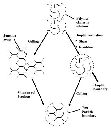
Figure 10 Schematic of gel particle formation mechanisms.
