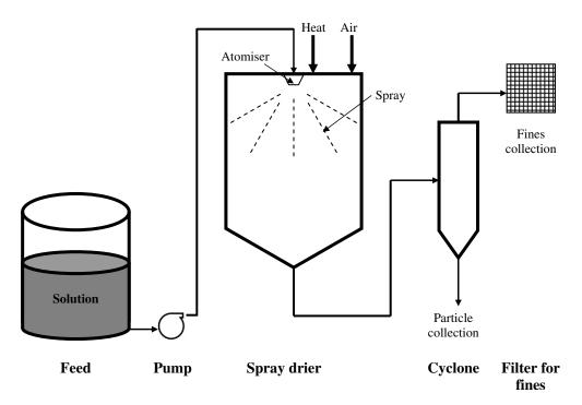
Figure 13 Schematic of the spray drying process.
