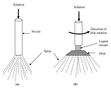
Figure 14 Schematic of a) nozzle atomization; b) disk atomization.
