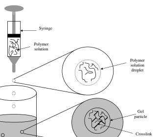
Figure 11 Extrusion formation of gel particles.
