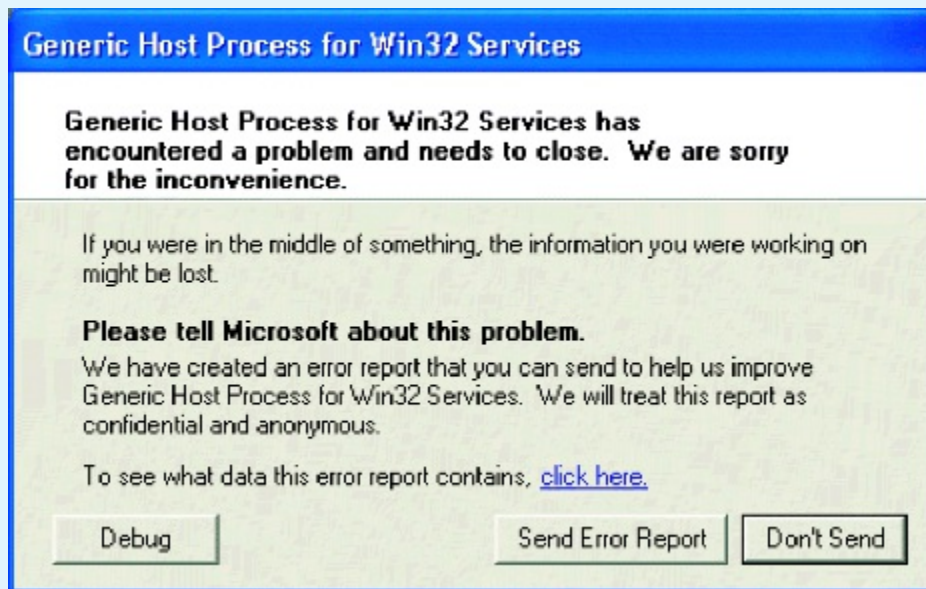
Figure 9.2 Two typical dialog boxes from the Windows error reporting system. This kind of reporting can have a significant effect on the quality of applications: for example, 29% of the errors fixed by the Windows XP (Service Pack 1) team were based on information collected through their ERS
