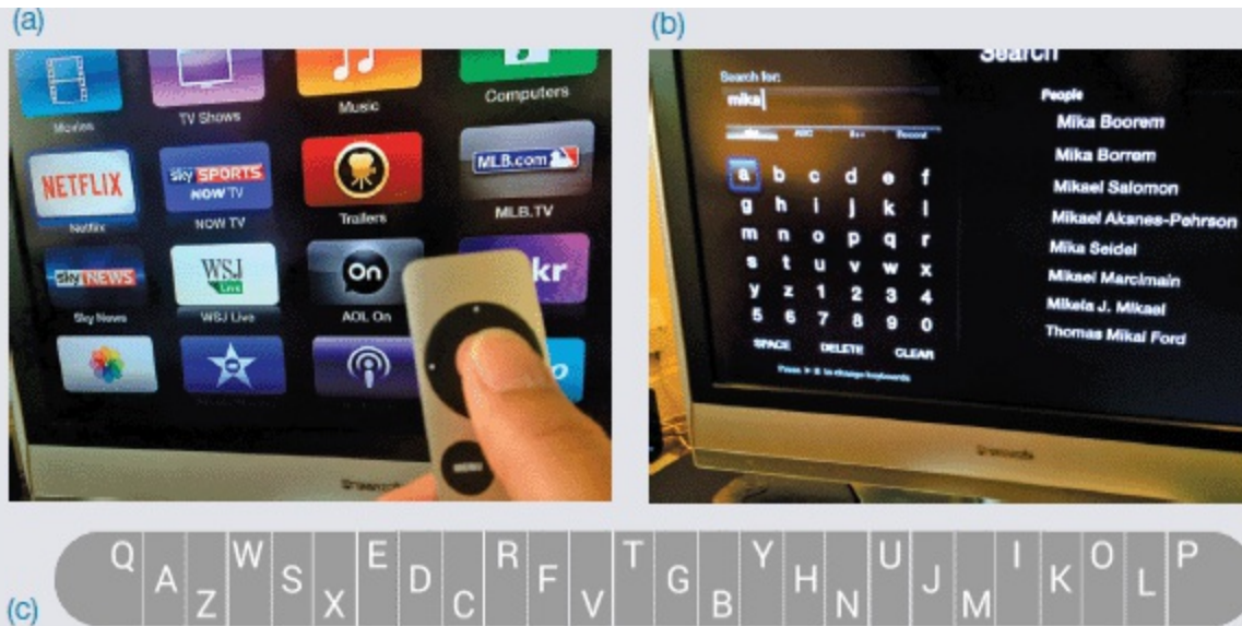
Figure 1.2 (a) Interacting with digital content on a TV screen using Apple TV remote controller (b) The online table of letters and numbers that the user has to select by pressing one button on the remote (c) Minuum's small staggered keyboard
