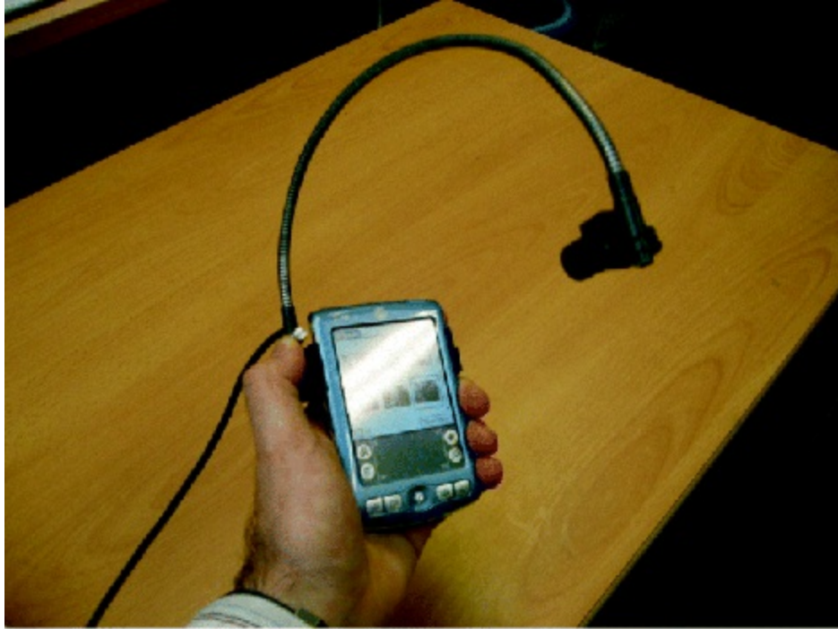
Figure 14.4 The Tracksys system being used with a mobile device camera that attaches to a flexible arm, which mounts on a mobile device, and is tethered to the lab
