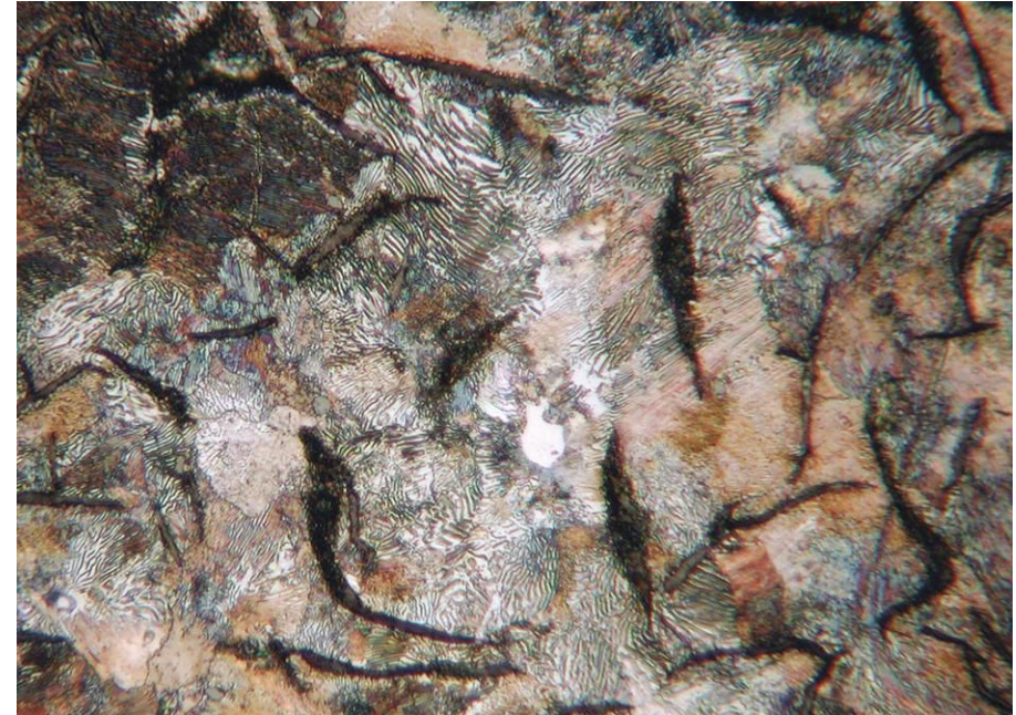
Fig. 2. Pearlitic Structure of a Cryogenically Treated Gray Cast Iron Brake Rotor: 100X, 2% Nital (Courtesy of Controlled Thermal Processing, Inc.)
