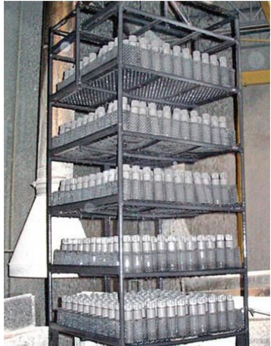
Fig. 8. Typical salt-bath-nitrided load
