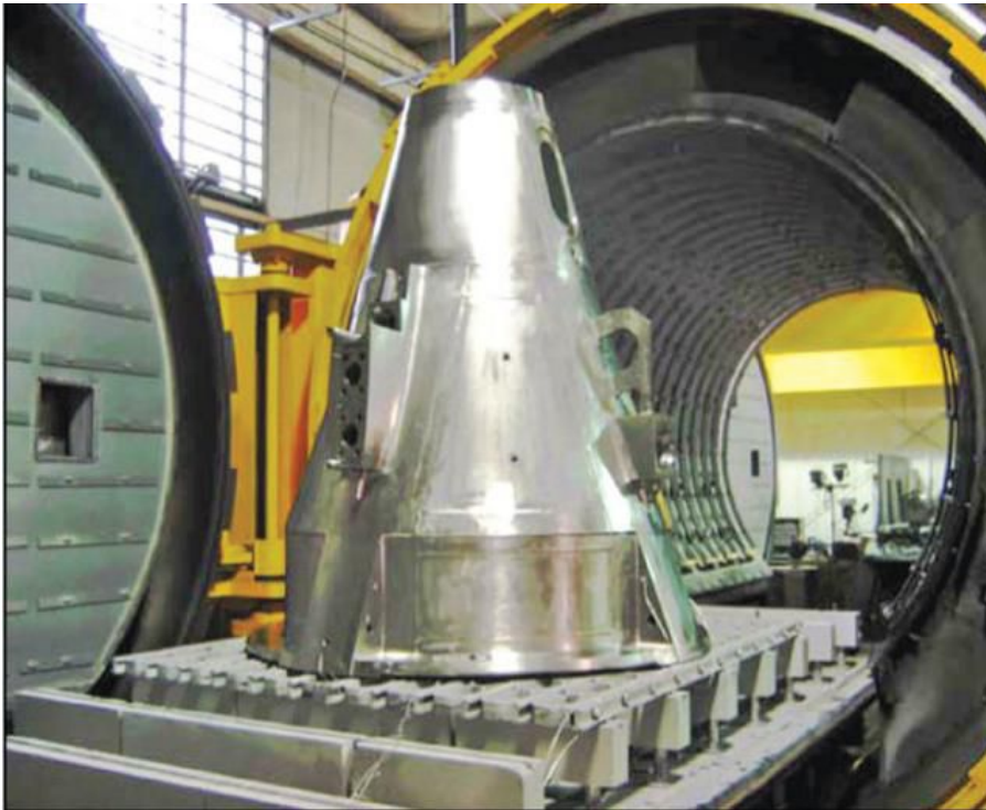
Fig. 3. Machined component ready for stress relief (Photograph courtesy of Solar Atmospheres, Inc.)
