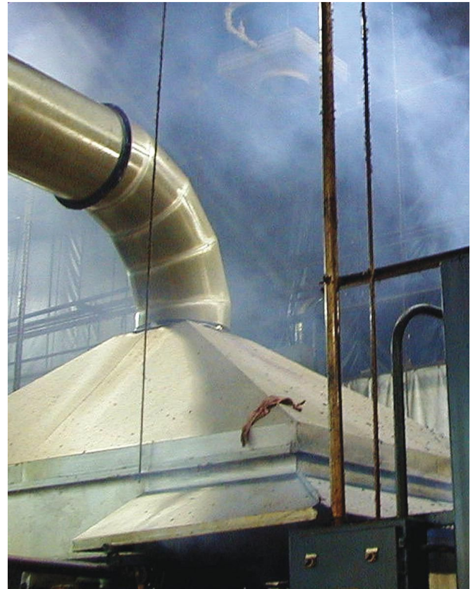
Fig. 3. Smoke generated from oily loads being tempered
