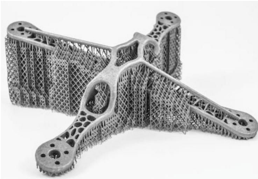
Fig. 2. A lightweight drone support structure created using AM [3]
