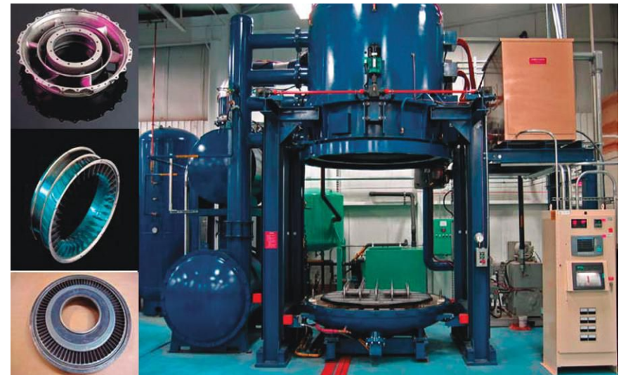
Fig. 1b. Various aerospace components brazed in a bottom-loading vacuum furnace
