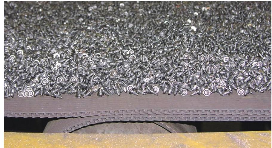
Fig. 4. Load of fasteners on a mesh belt for carbonitriding
