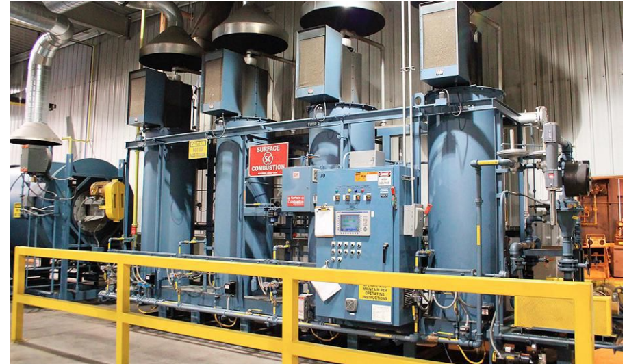
Fig. 3. Modular multi-retort endothermic gas (Rx®) generator (courtesy of Surface Combustion, Inc.)
