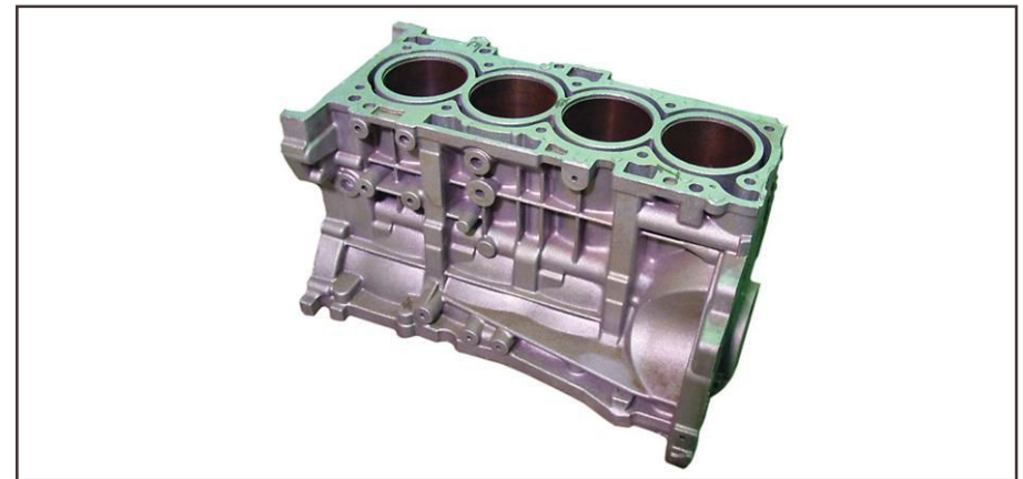
Fig. 1. Cast aluminum engine block (Photograph Courtesy of Wisconsin Oven Corporation; East Troy, Wis.)
