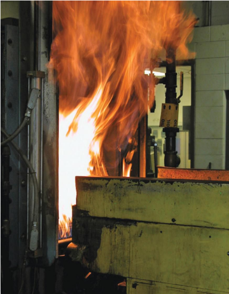
Fig. 1. Properly adjusted furnace flame curtain
