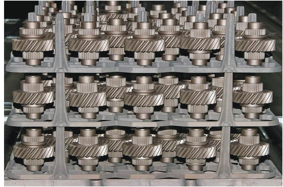
Fig. 5. Typical LPC vacuum-carburized components (Photograph courtesy of ALD Thermal Treatment)
