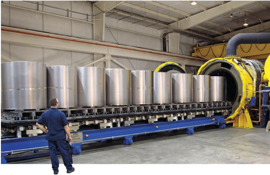
Fig. 2. Vacuum annealing of titanium coils. (Photograph courtesy of Solar Atmospheres)
