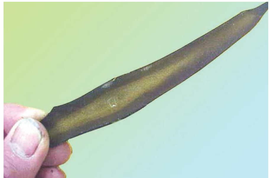
Fig 1. Exfoliated steel sliver
