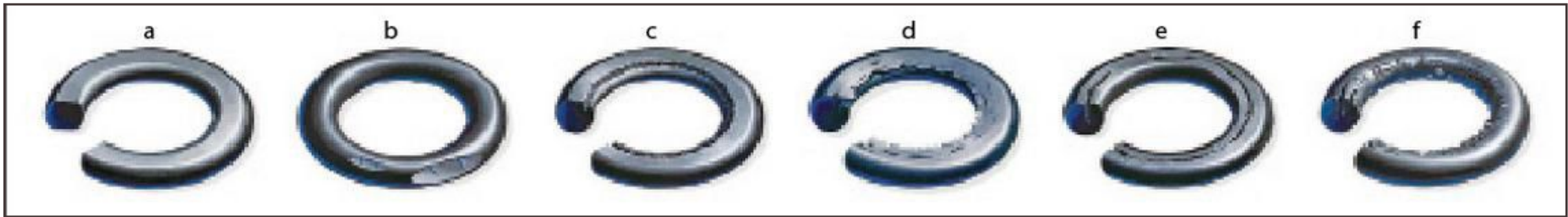
Fig. 5. Typical O-ring failures [3]
