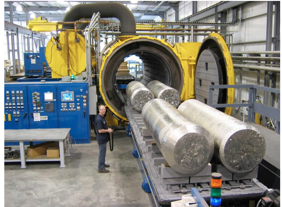
Fig. 9. Vacuum homogenizing of titanium ingots (Photograph courtesy of Solar Atmospheres)
