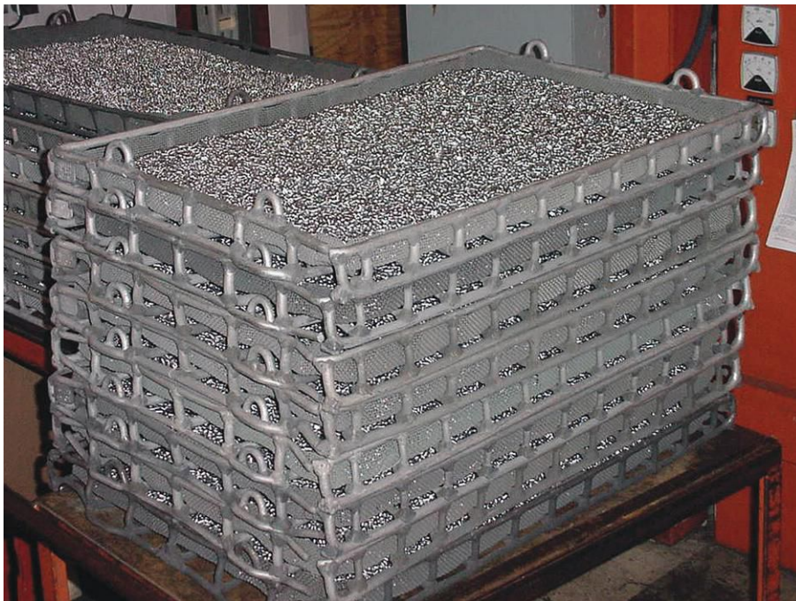
Fig. 2. Typical load of 17Cr-4Ni fasteners for vacuum heat treatment (courtesy of Solar Manufacturing)
