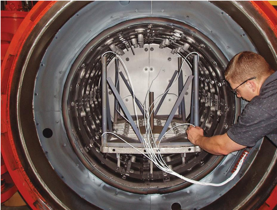
Fig. 1. Single-chamber vacuum furnace temperature-survey rack in position (Photograph courtesy of Solar Atmospheres Inc.)
