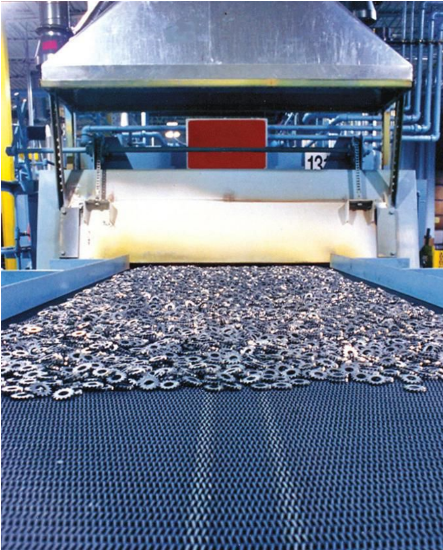
Fig. 1. Typical mesh-belt-furnace part loading (Courtesy of Surface Combustion, Inc.)
