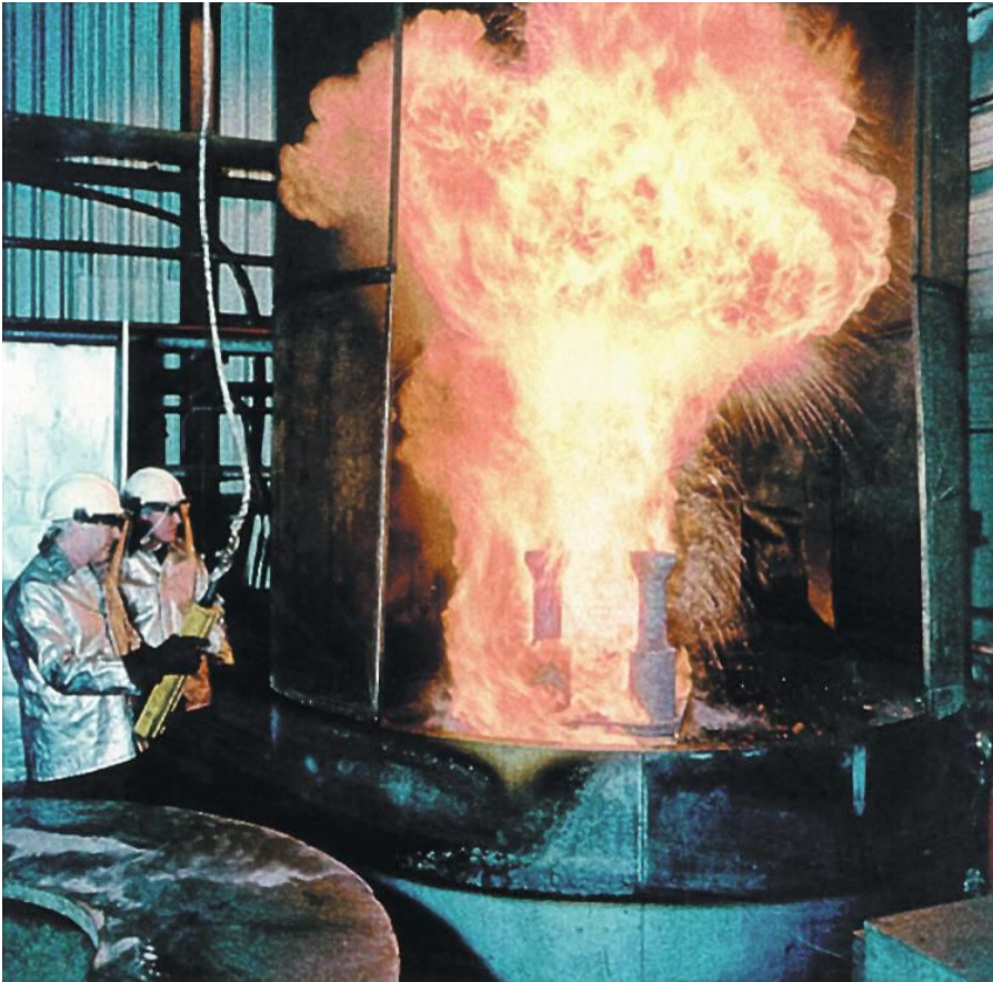
Fig. 2. Quenching into an oil tank
