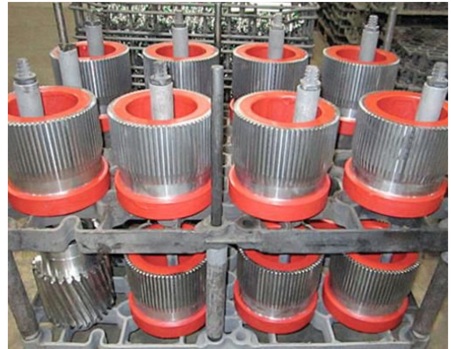
Fig. 3. Typical commercial heat-treat load of gears for vacuum carburizing. (Photo courtesy of Midwest Thermal-Vac)
