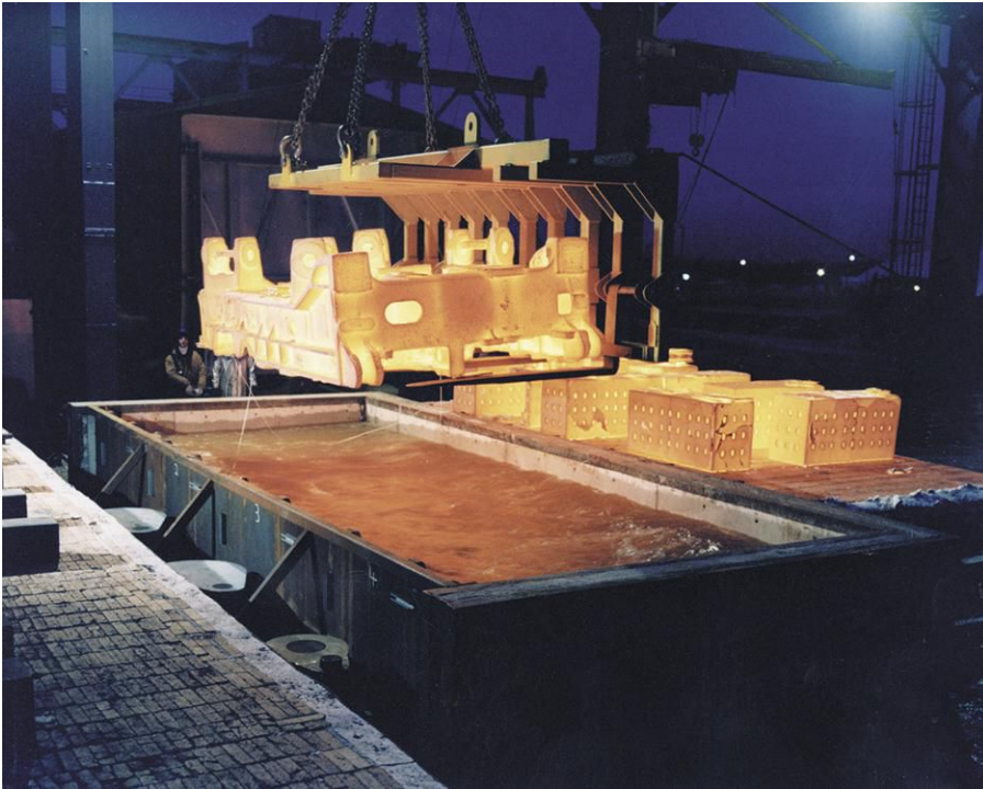
Fig. 1. Quenching into a polymer tank
