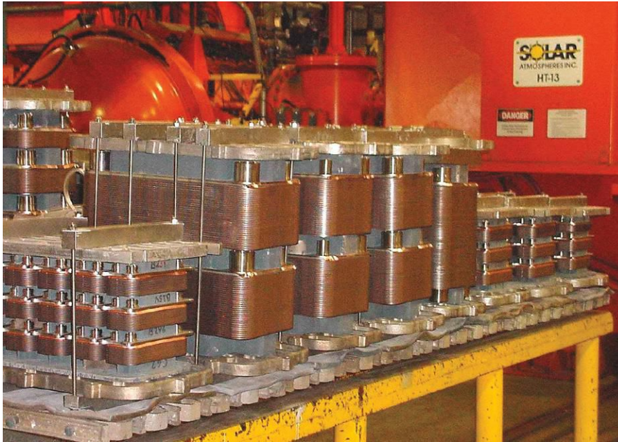
Fig. 1 Load of flat-plate heat exchangers ready for processing under partial pressure. Photo courtesy of Solar Atmospheres Inc, Souderton, Pa.
