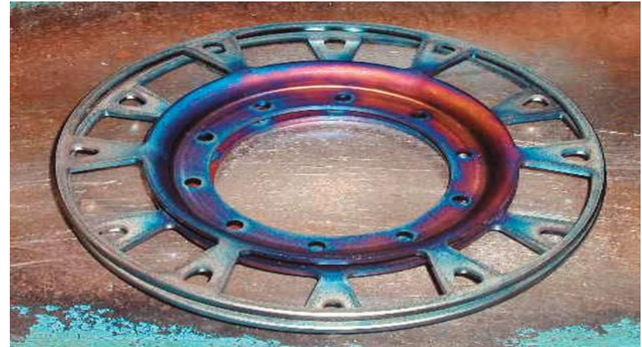
Fig. 1. Example of tempering color variation (support plate)
