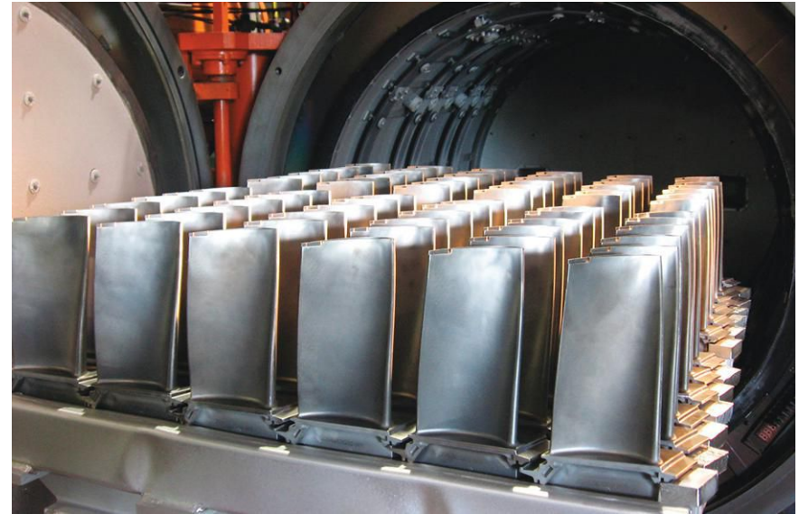
Fig. 1a. Jet engine turbine blades brazed in a horizontal vacuum furnace
