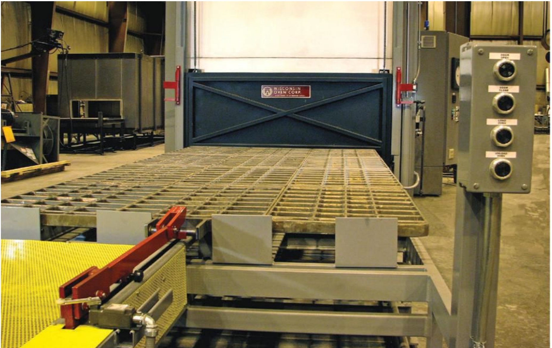
Fig. 1. Typical heat-treat processing oven (Photograph courtesy of Wisconsin Oven Corporation)
