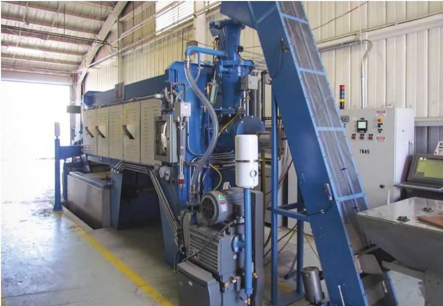
Fig. 6. Electrically heated shaker-hearth furnace for titanium fasteners (courtesy of DF Industries, Inc.)
