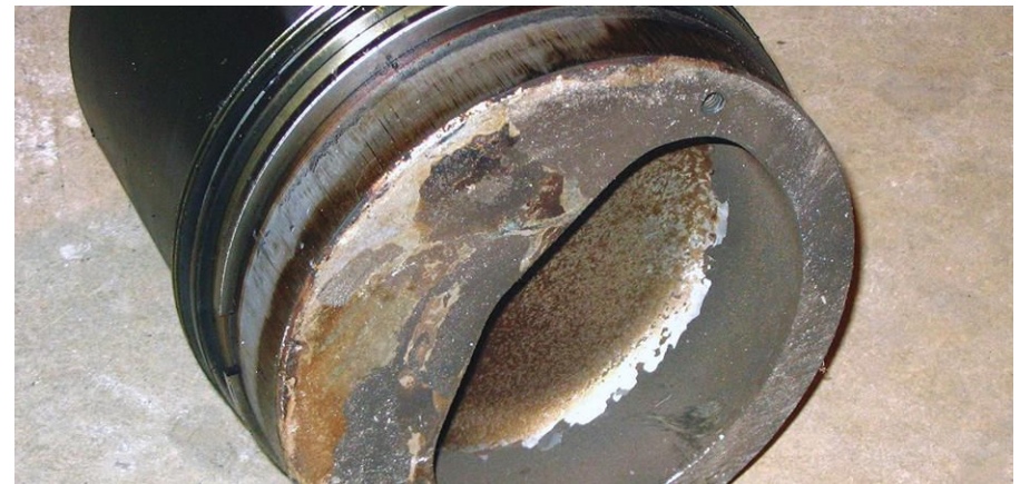
Fig. 2. Piston head component from failed power generation engine (photograph courtesy of Materials Engineering Inc.)
