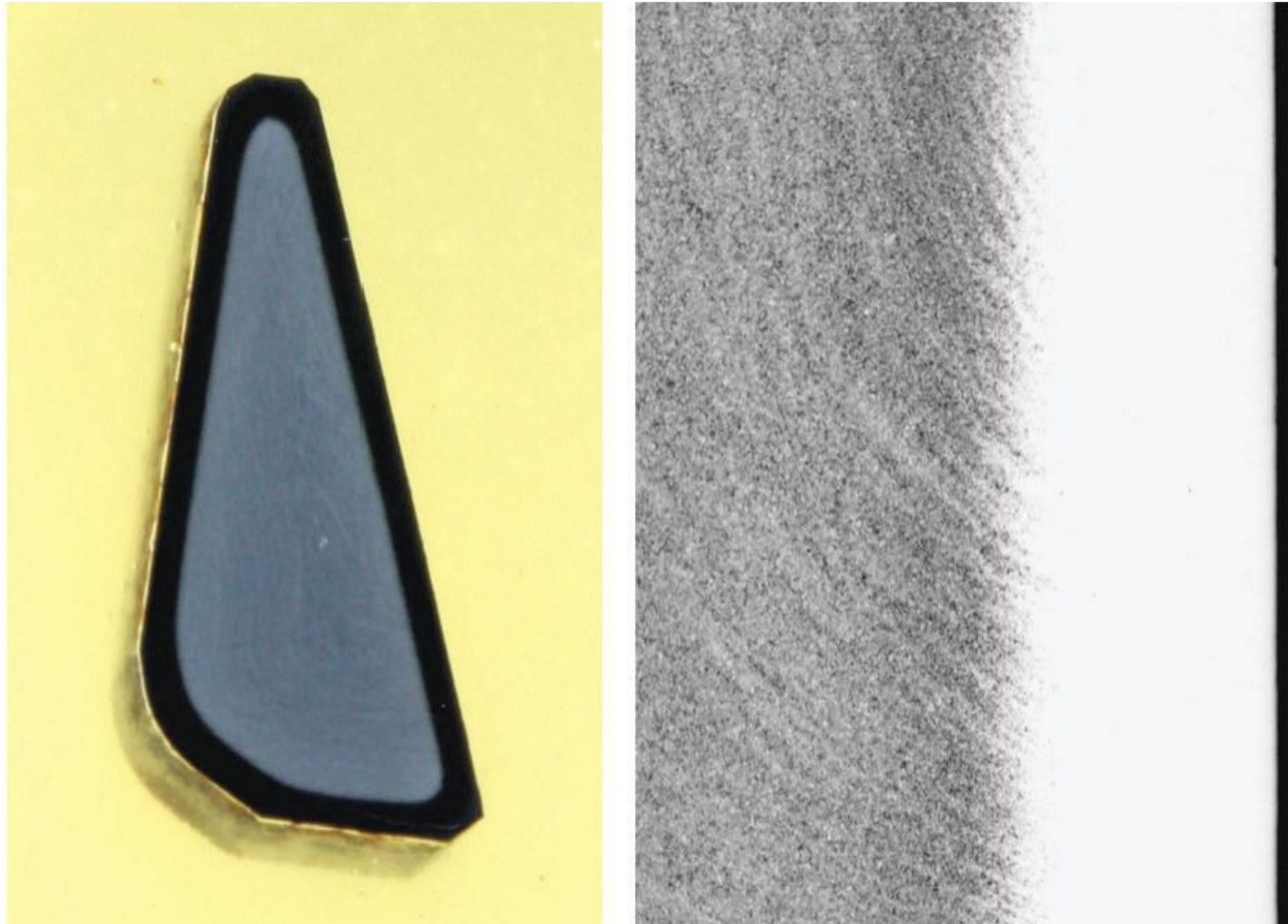
Fig. 1. Case/core demarcation by Ms point method (0.50% C sample) (a) Ms test specimen (2-3X) that has been heat treated, mounted, polished and etched. The lighting makes the unetched (fresh martensite) zone on the outer edge look black, but it is actually a shiny polished surface. (b) Close-up of the demarcation zone between the etched (tempered-martensite) zone and the unetched (fresh-martensite) zone. The line of demarcation is not exact. Generally, the depth is “read” using a Brinell scope at approximately 12-15X. When you read the depth, you read to the depth where the tempered martensite layer is consistent (not to the outer edges of the tempered martensite wisps). At 12-15X the line is not as fuzzy and the depth can be pretty consistently measured to \pm 0.001 inch (0.025 mm) or so.
