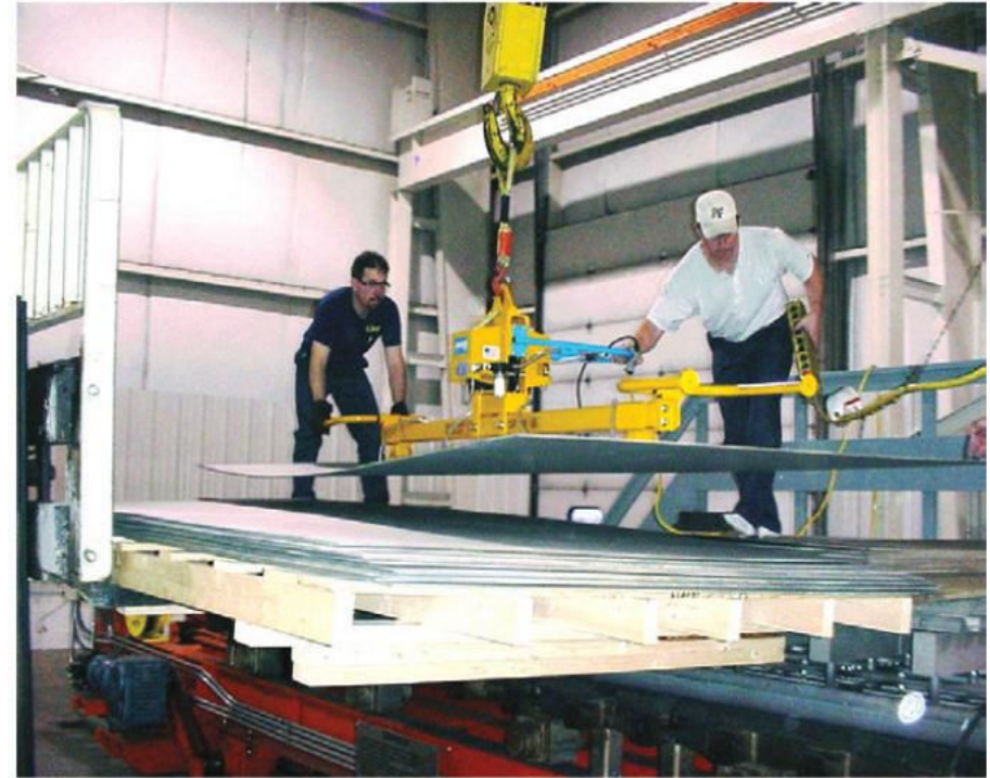
Fig. 2. Load of titanium sheet for vacuum age hardening (Photograph Courtesy of Solar Atmospheres of Western Pennsylvania)
