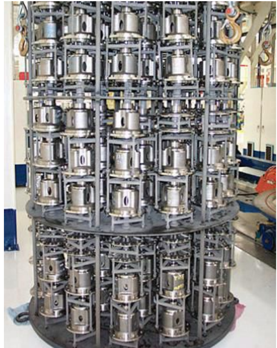
Fig. 6. Typical gas-nitrided load
