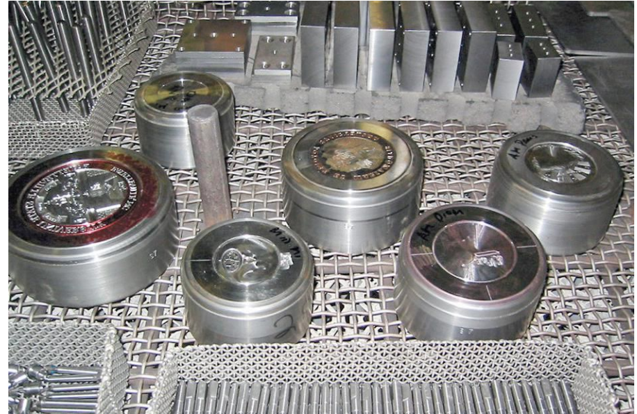
Fig. 2. Typical tool-and-die parts being prepared for heat treatment
