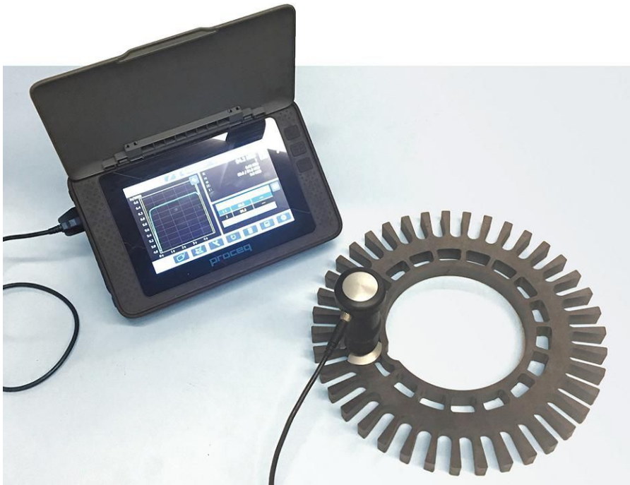
Fig. 2. Change “Portable ... tester” to read “Equotip 550 display unit compatible with 3 hardness test methods - Leeb (rebound), UCI (Ultrasonic Contact Impedance), and Portable Rockwell Hardness (shown above)” (courtesy of Columbia Machine Inc.)
