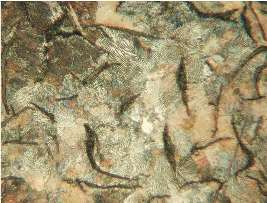
Fig. 7. Pearlitic structure of a cryogenically treated gray cast-iron brake rotor; 100X; 2% nital etch (courtesy of Controlled Thermal Processing Inc.)
