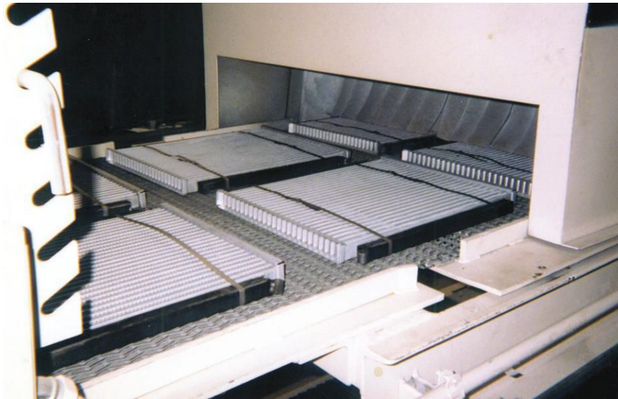
Fig. 2 CAB brazed aluminum heat exchanger assembly. Courtesy of SECO/WARWICK Corp.
