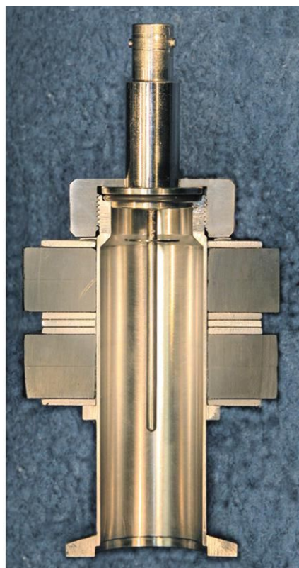
Fig. 10. (left) Cold-cathode gauge [3] Fig. 11. (right) Cross-sectional view of a cold-cathode gauge [3]
