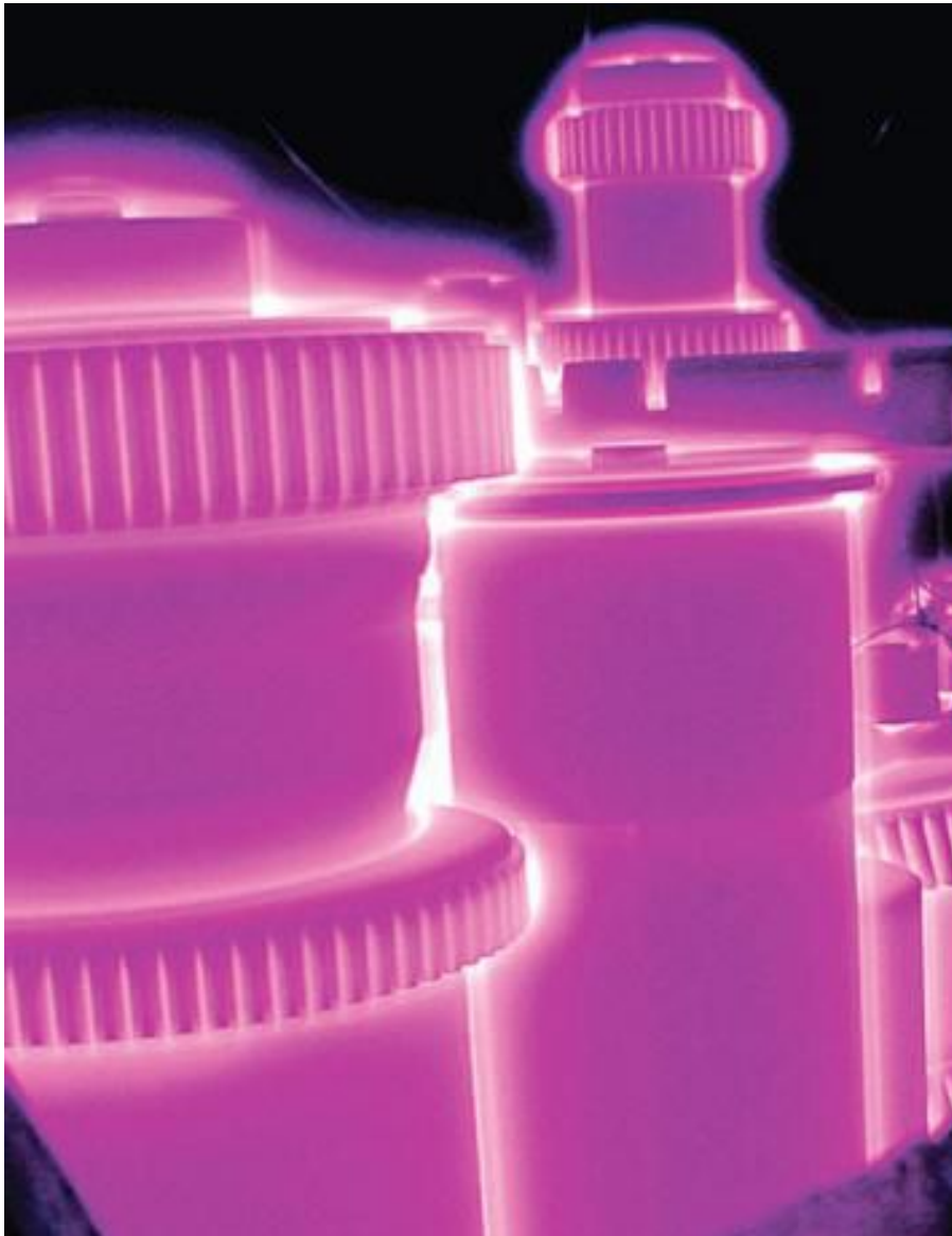
Fig. 7. Typical plasma-nitrided load
