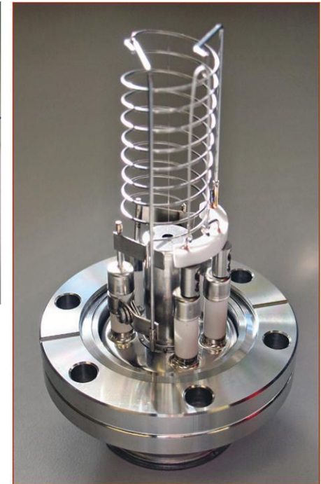
Fig. 8. Bayard-Alpert ionization gauge [3]
