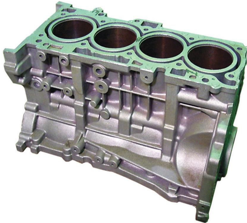
Fig. 2. Magnesium casting after solution treating
