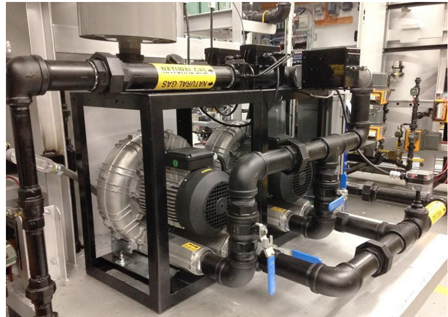
Fig. 6. Endoinjector® fuel-injection gas mixing system mounted on an endothermic gas generator (courtesy of Atmosphere Engineering Company)
