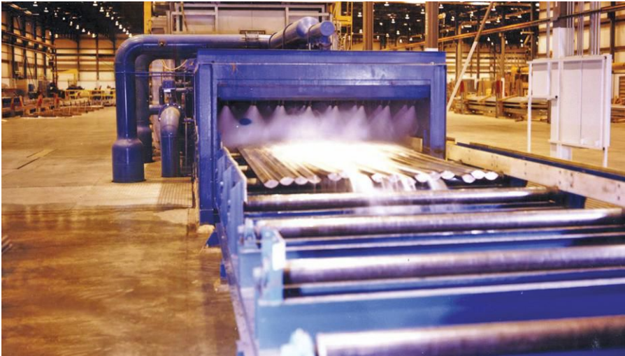
Fig. 1. Alloy bar stock exiting a roller hearth furnace. (Photo Courtesy of SECO/WARWICK Corporation)
