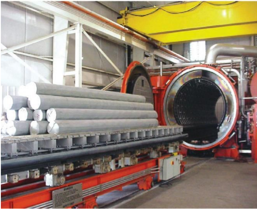
Fig. 3. Load of titanium ingots for vacuum degassing (Photograph Courtesy of Solar Atmospheres of Western Pennsylvania)
