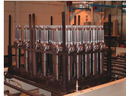
Fig. 4. Heavy-duty truck shafts low-pressure vacuum carburized and oil quenched
