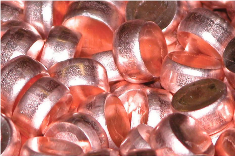
Fig. 1 Vacuum annealing of copper heat sink blanks
