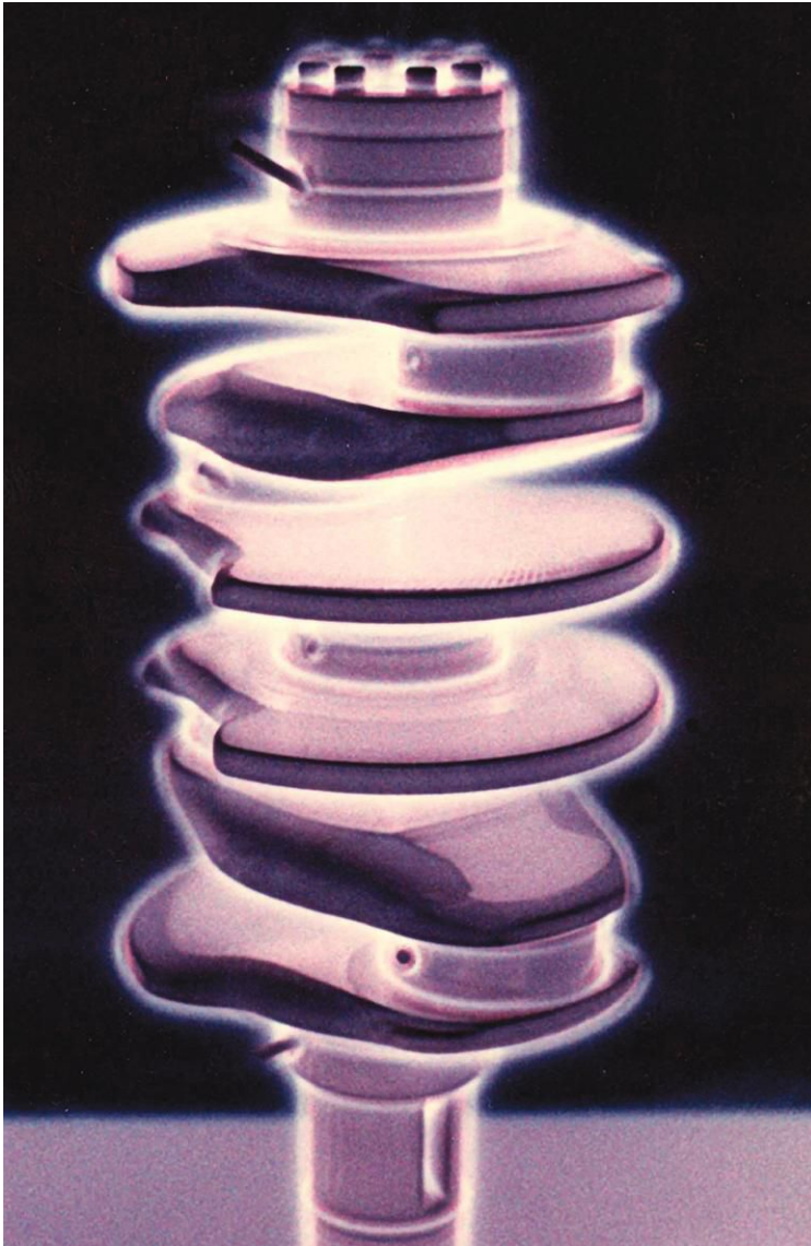
Fig. 6. Plasma nitriding of automotive crankshafts (Photograph Courtesy of Surface Combustion)
