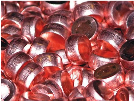
Fig. 6. Bright annealing of copper diodes for heat sinks
