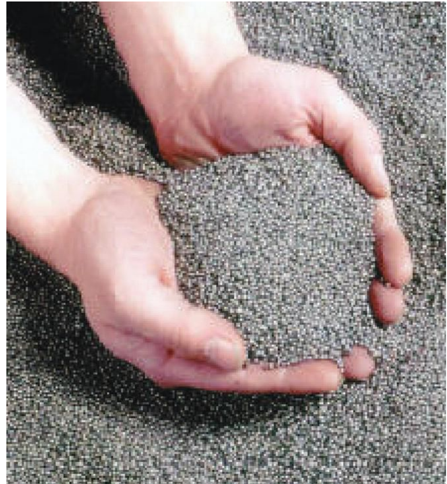
Fig. 1. Abrasive shot blast media (photograph courtesy of Eisenwerk Würth GmbH, www.eisenwerk.com )
