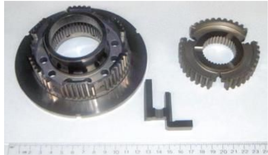
Fig. 6. Clutch and synchronizer hubs after LPC+HPGQ – SL-5506 material (Photograph courtesy of Stackpole Ltd.)
