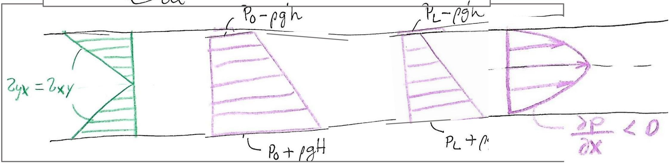
$$\langle v_x \rangle = \frac{1}{2HW} \cdot \int_{-H}^H \int_0^w a(y^2 - H^2) dz dy = \frac{w}{2HW} \cdot a \int_{-H}^H (y^2 - H^2) dy$$
