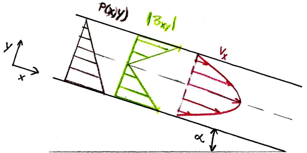
$$\vec{\sigma} = \begin{bmatrix} \sigma_{xx} & \sigma_{xy} & \sigma_{xz} \\ \sigma_{yx} & \sigma_{yy} & \sigma_{yz} \\ \sigma_{zx} & \sigma_{zy} & \sigma_{zz} \end{bmatrix} = \begin{bmatrix} 0 & \frac{\rho g \sin \alpha}{2} (D-2y) & 0 \\ \frac{\rho g \sin \alpha}{2} (D-2y) & 0 & 0 \\ 0 & 0 & 0 \end{bmatrix}$$
