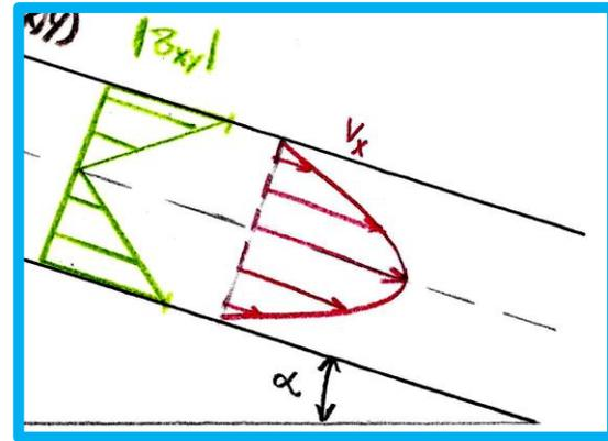
$$v_x = -\frac{\rho g \sin \alpha}{\mu} \frac{y^2}{2} + C_1 y + C_2$$
