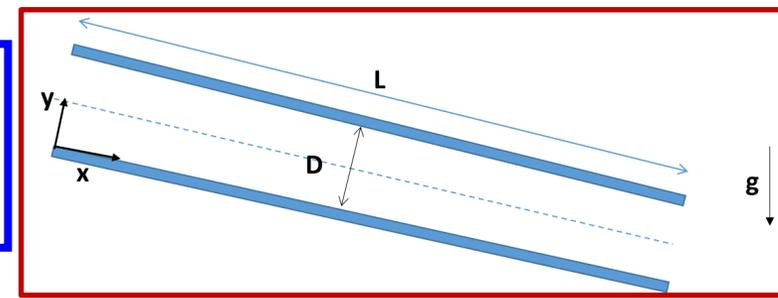
$$\rho g_x + \mu \frac{\partial^2 v_x}{\partial y^2} = 0 = \rho g \sin \alpha + \mu \frac{d^2 v_x}{dy^2}$$
