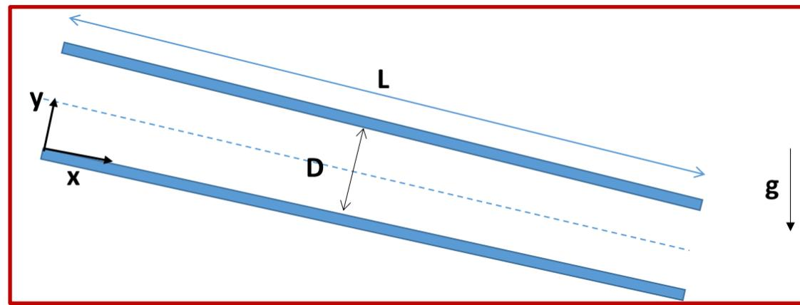
$$\rho \frac{D\vec{v}}{Dt} = \rho \frac{\partial \vec{v}}{\partial t} + \rho \vec{v} \cdot \text{grad} \vec{v} = \rho \vec{g} - \text{grad} p + \mu \text{lap} \vec{v}$$
