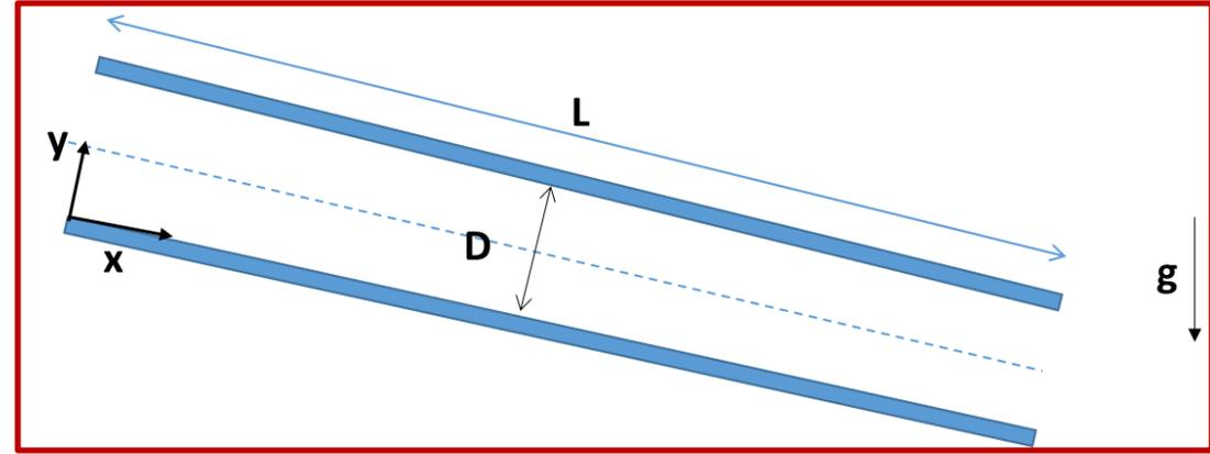
$$\rho \frac{D\vec{v}}{Dt} = \rho \frac{\partial \vec{v}}{\partial t} + \rho \vec{v} \cdot \text{grad} \vec{v} = \rho \vec{g} - \text{grad} p + \mu \text{lap} \vec{v}$$
