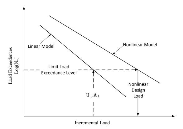
Figure 5. Establishing Limit Load for a Nonlinear Airplane
