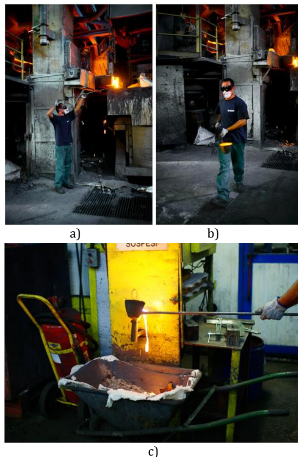
Fig. 1. Different phases of chemical inspection during the processing: a) molten metal extraction; b) manual transport; c) spilling on the instrument for the detection of chemical elements.
