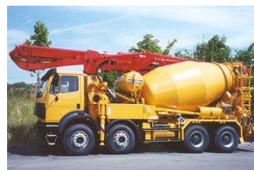
Putzmeister PUMI, concrete ready mix truck & pump combined, Munich
