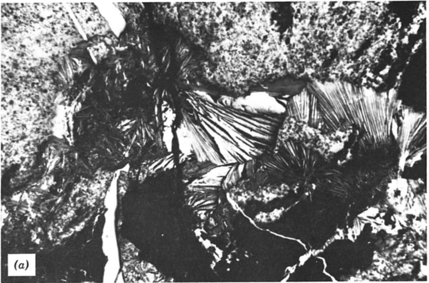
FIGURE 7.9 (a) Radiating fibrous crystals of the manganese oxide mineral chalcophanite infilling an open fracture, Red Brush Mine, Virginia (width of field = 2,000 \mu\text{m} ). (b) Radiating clusters of fibrous goethite crystals forming a botryoidal aggregate in a weathering zone, Giles Co., Virginia (width of field = 2,000 \mu\text{m} ).
