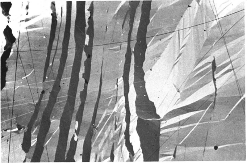
FIGURE 7.21 Complex pressure lamellae developed in stibnite as a result of deformation; the wide variety of colors results from different crystallographic orientations of the lamellae; crossed polars (width of field = 520 \mu\text{m} ).
