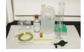
Add 1 part acid to 4 parts distilled water in the graduated cylinder and mix throughly with the glass rod. Caution: acetic acid can cause burns. Wear safety goggles, plastic gloves, and an apron while working with this chemical.
