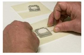
Additional sample can be used as filler if necessary to create a firm pack. This part of the sample need not be as finely ground, as it will become the bottom surface and will not be exposed to the X-ray beam.
