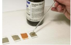
Mounts are ready to be X-rayed as soon as liquid is uniformly absorbed. Excess ethylene glycol may be gently mopped up with lab tissue.
