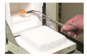
Remove mount by pulling it forward with the wire hook until the edge of the mount can be grasped with the tongs. Do not remove mounts until they are ready to be run on the diffractometer.
