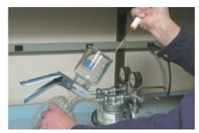
As soon as the remaining suspension has been completely drawn into the filter, remove the glass funnel and use a single-edge razor or metal spatula to remove the moist filter from the filtering device.
