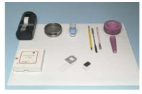
Tape the glass slide over the opening of the sample holder. Leave tabs on each side for later removal of this cover, but fold the extra tape against itself so that it will not stick to other objects or the sample. Place the holder glass side down on a piece of weighing paper.
