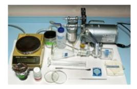
Weigh out 9.5 g of LiCl for each 100 ml of distilled water used to make the solution. Dissolve the LiCl in the glass jar by stirring with the glass rod to make up a 3N solution of lithium chloride.
