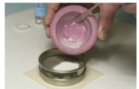
Brush the sample through the sieve into the cavity of the sample holder. The purpose of the brushing is to obtain an even distribution and to minimize preferred orientation of the particles.
