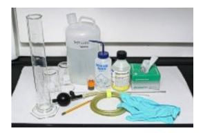
If the hydrogen peroxide is laboratory grade (30%), prepare a dilute solution of 3% using a graduated cylinder and distilled water. Caution: hydrogen peroxide is a strong oxidizer that can cause severe burns. Wear goggles, plastic gloves, and an apron while working with this chemical.
