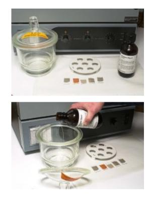
Place oriented aggregate mounts on the shelf of desiccator. Additional shelves may be stacked if necessary.
