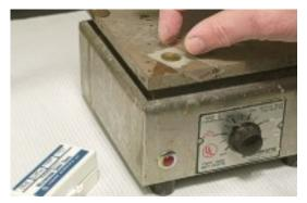
Press the cover slip down with a pair of tweezers. The Piccolyte should spread to fill the space beneath the cover glass.
