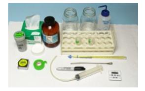
Label the jars with 0 and 5-cm depths. Sample identifiers should be labeled on the jars and centrifuge tubes with labeling tape for easy removal later.
