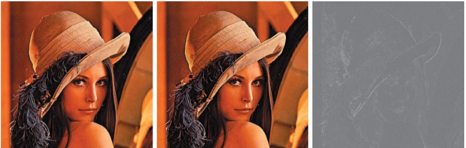
FIGURE 6.41 Image sharpening with the Laplacian. (a) Result of processing each RGB channel. (b) Result of processing the HSI intensity component and converting to RGB. (c) Difference between the two results.
