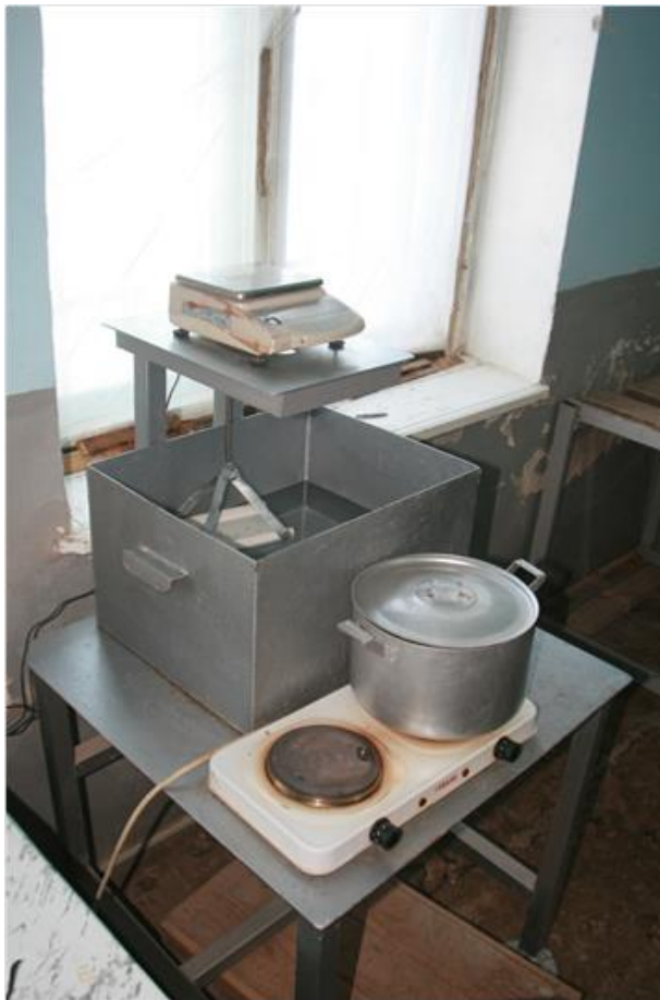
Figure 11-1: Station for Measuring Dry Bulk Density at Gorayk Core Shed Facilities
