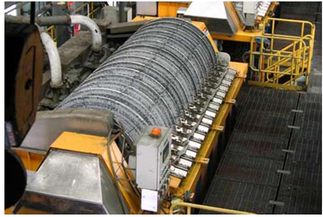
FIG 13.23 - Ceremec disc filter (source: Larox Pty Ltd).
