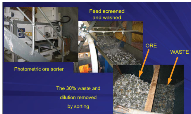
FIG 12.20 - Colourimetric ore sorting machine.
