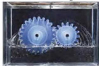
v_t = 0.88 m/s IOL = pinion pitch radius
