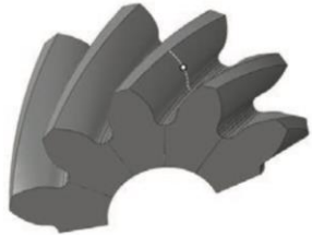
Fig. 1 – Finite Element Model of the helical gears: a) numerical model of five pairs of helical gear tooth, in which blue indicates the near surface region while the light gray indicates the bulk region of gear teeth; b) central point and path of numerical results extraction.
