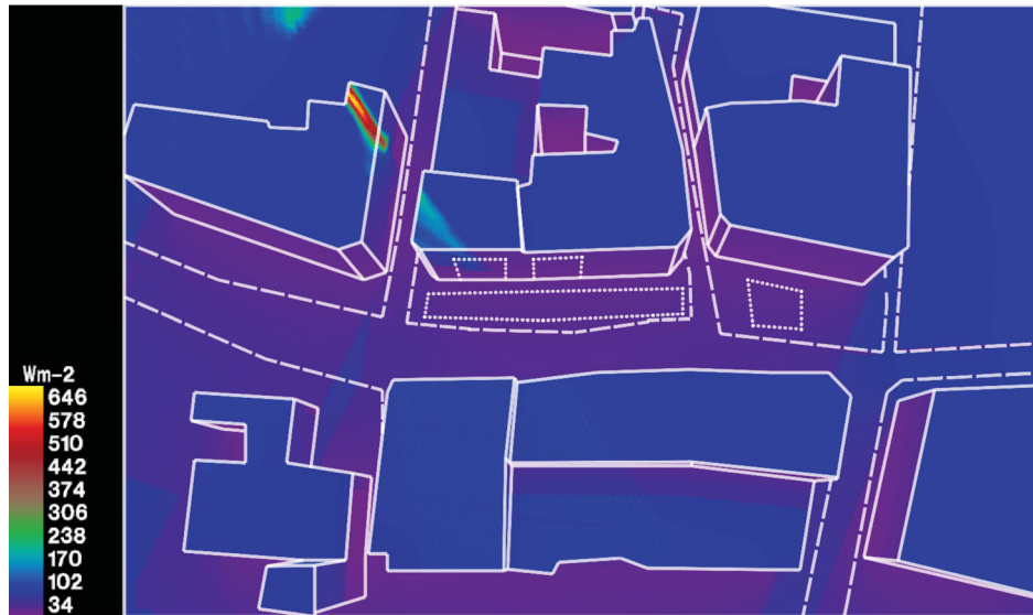
Figure 9. Heat flux predictions for 13:40 pm on 12th of October using an intermediate sky model.
