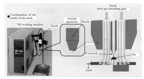
Figure 3. Principle of TIG welding.
