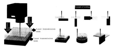
Figure 2. How resin welding works.
