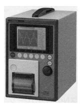
Photo 3. Micro-resistance welding monitoring device (Checker) [MM-370A].
