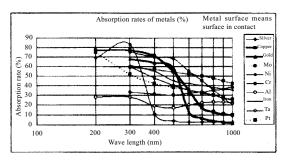
Figure 1. Absorption rates of metals.
