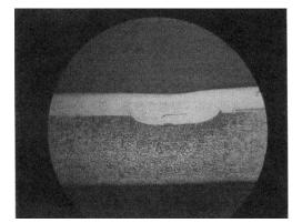
Photo 1. Cross sectional photo of micro-resistance weld (Nickel (0.15 mm) × nickel-plated iron (0.35 mm thick)).
