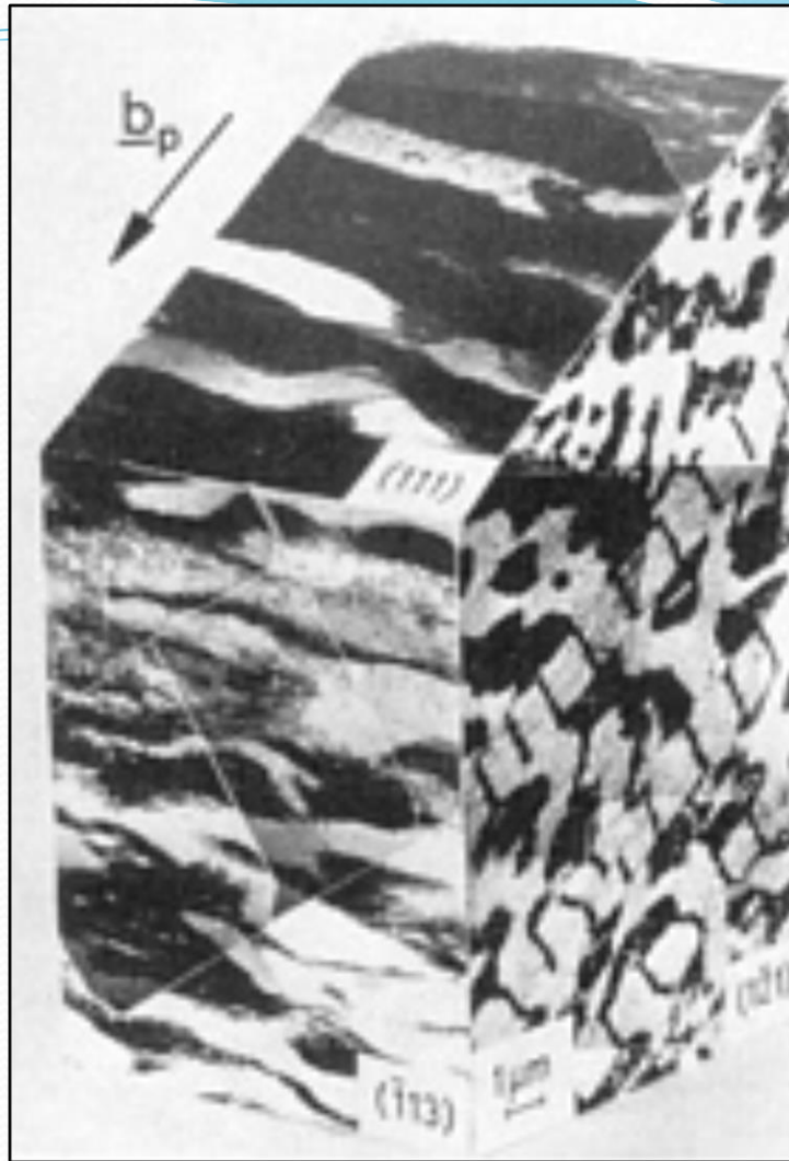
Typical ladder-like structure of PSBs (Metals Handbook, vol. 19)
