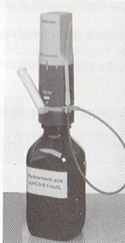
Dosino The buret motor is directly placed onto the reagent bottle. Used for automatic titrators.
