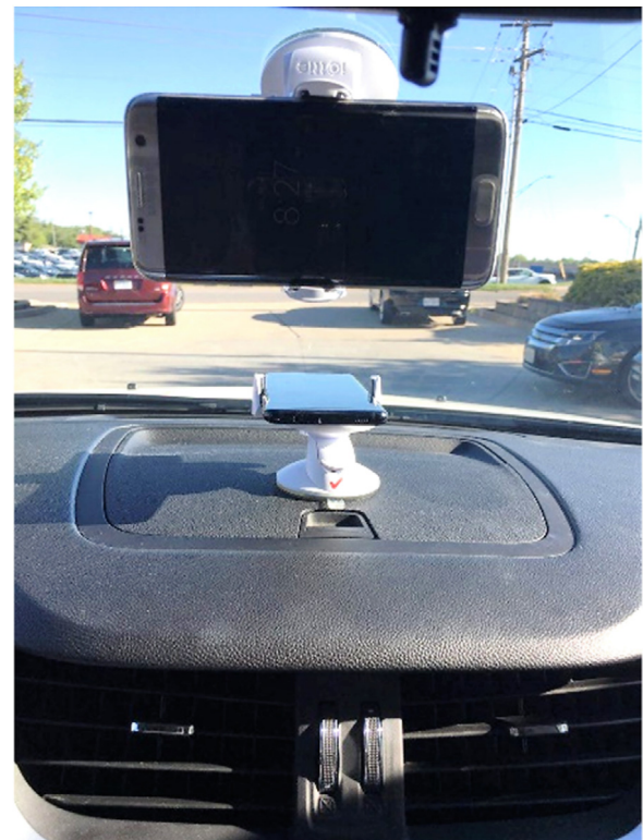
Fig. 31. The smartphone mounting arrangement.
