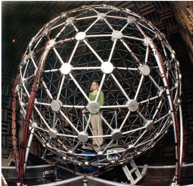
Figure 12.2 ■ In this sound localization tester at Wright-Patterson AFB in Dayton, Ohio, the listener is surrounded by 227 loudspeakers. (Courtesy of Marc Ericson, Wright-Patterson Air Force Base, Dayton, OH.)
