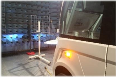
The AUTONOM shuttle, radiation emission setup
