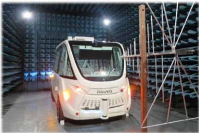
The AUTONOM shuttle, radiation immunity
