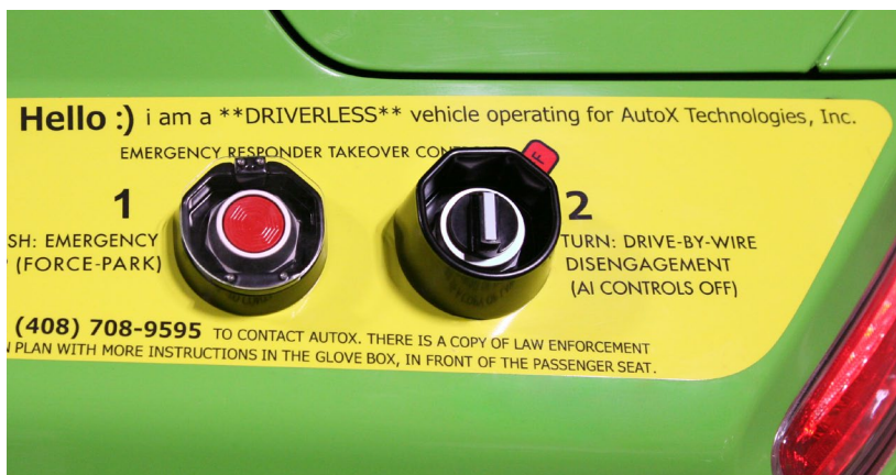
Exterior emergency button and A.I. control disengagement switch
