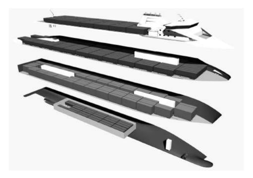
Figure 18: Enclosed and open cargo spaces
