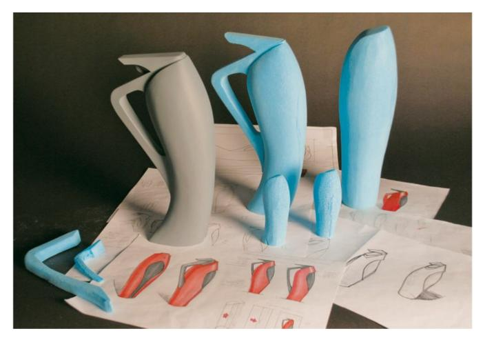
Industrial design prototypes are used for iterative form development, gauging user response, and communication of design concepts.
