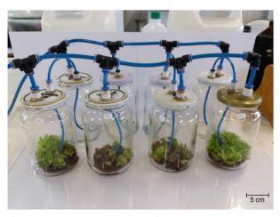
**Figure 1:** Bioreactor with dual container system (500 mL capacity).
