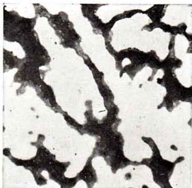
Fig. 8-8. Cast Pt + 60% Ag hyperperitectic alloy. White and light gray areas are residual cored \alpha ; dark two-toned areas are \beta , the outer portions being of peritectic composition and the darkest central areas being the cored \beta that formed at temperatures below that of the peritectic reaction. Magnification 1,000.
