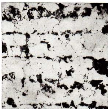
FIG. 11-7. Binary steel, 0.3% C, showing banding of the eutectoid constituent resulting from dendritic segregation. Magnification 100.
