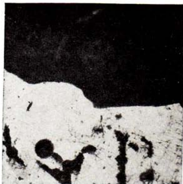
FIG. 10-3. Microstructure at the junction between the two layers in a cast "alloy" composed of equal parts of sodium and zinc. The lower layer is the \beta (compound) phase; the upper layer is nearly pure sodium. Dark spots in the \beta layer are inclusions of sodium. Magnification 75.
