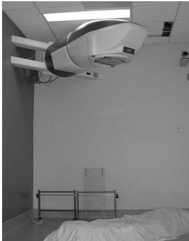
FIG. 15.5. A cobalt-60 teletherapy unit dedicated for total body irradiation. The source-floor distance is 250 cm, the patient is treated on a floor mattress in a prone and supine position to obtain a parallel-opposed beam.
