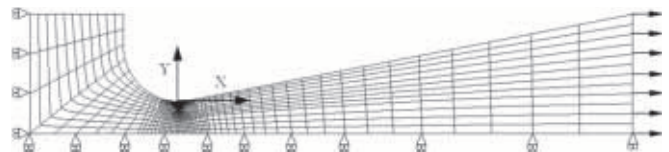
Fig. 2. Washer specimen 2D FE model for stress analysis.
