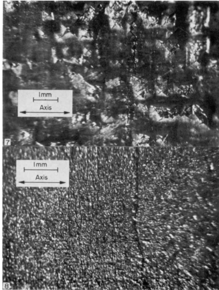
Fig. 7. Torsional zig-zag cracks. Series 2, \Delta\gamma = 1.75\% . Fig. 8. Torsional Stage I cracking. Series 2, \Delta\gamma = 7.8\% .
