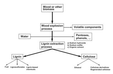
**Figure 8.3.** Principal scheme for the "wood explosion" process and the types of products that can be obtained. Typical reaction conditions are 190–240 °C, 1–5 min.
