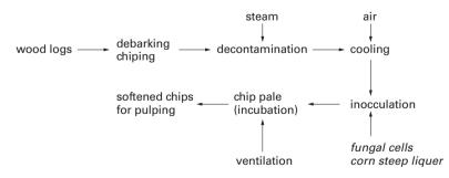
Figure 12.3. Overview of the basic components of a biopulping operation. Details of the process may vary depending on the conditions and facilities in particular mills.
