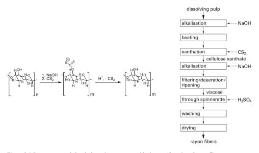
Figure 8.6. Process steps and chemical reactions encountered in the manufacturing of rayon fibers.
