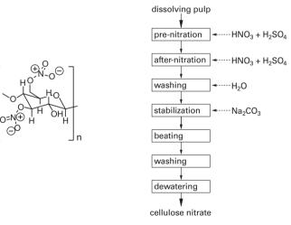
Figure 8.10. Process steps in the manufacturing of cellulose nitrate together with a simplified chemical structure.
