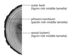
**Figure 12.6.** Principle for microbial aided barking. The Phloem and cambium layers (inner bark) located between the wood (xylem) and the other bark in wood are only lignified to limited extend and can therefore be degraded by moulds.
