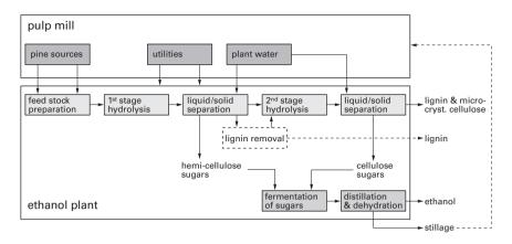
**Figure 8.18.** Suggested production unit for conversion of wood waste to ethanol using the CASH process employing sulfur dioxide and sulfuric acid in two stages. The integration with a pulp mill is indicated in the figure.
