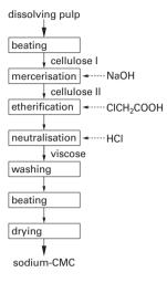
Figure 8.8. Process steps in the manufacturing of carboxymethylcellulose (CMC) together with a simplified chemical structure of CMC.
