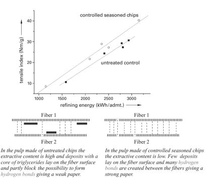
**Figure 12.5.** Effect of controlled seasoning on paper strength of thermomechanical Scots pine pulp. The graph above shows that the tensile strength is higher at similar refining energy for controlled seasoned chips than the untreated control. Thus a fungal pretreatment may save energy, or alternatively produce a stronger paper. The cartoon below shows a hypothesis for the mechanism behind the effect. For a discussion of the complex strength developments in mechanical pulp, see Volume 2.
