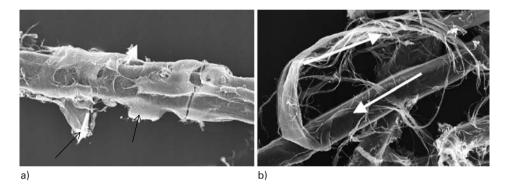
**Figure 3.18. Importance of the wood cell wall layers in pulping.** a) When wood fibres are refined the primary wall is often removed and the S1 layer becomes fibrillated (arrows); b) If refining is severe, fibrillation may also occur within the S2 layer. The orientation of fibrillation (arrows) reflects the MFA of the original wall layer.
