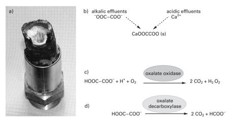
**Figure 12.16.** Enzymes degrading oxalic acid a) spray pipe with calciumoxalate precipitation. b) Principle behind precipitation. c) degradation of oxalic acid with oxalate oxidase d) Degradation of oxalic acid with oxalate decarboxylase.
