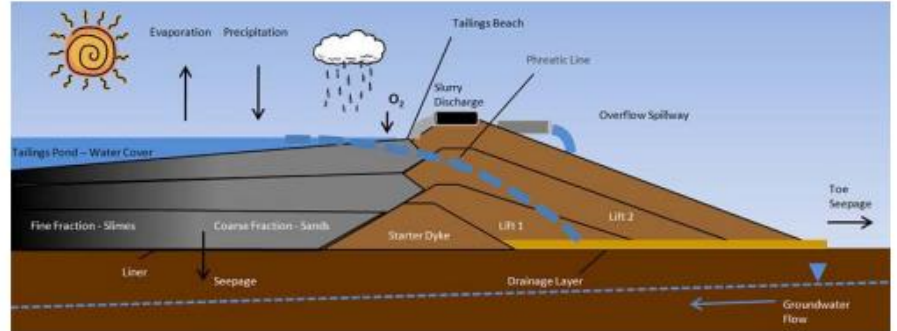
Centerline Raise Construction Method
