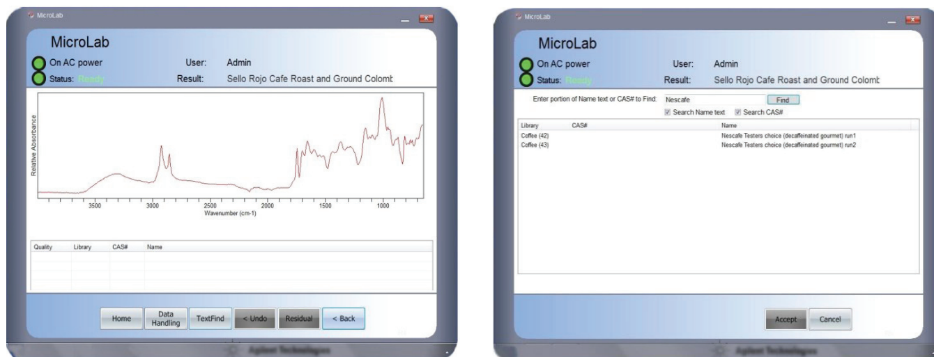
Figure 12. Unknown coffee sample is identified by automated matching of its spectra with reference spectra in the on-board library
