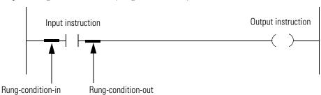
Only input instructions affect the rung-condition-in of subsequent instructions on the rung.
