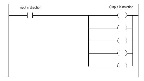
You can nest branches to as many as 6 levels. This example shows a nested branch. The bottom output instruction is on a nested branch that is three levels deep.
