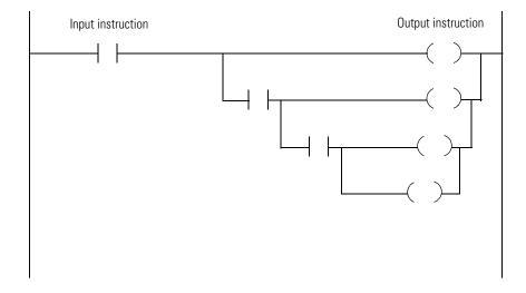
Large rungs with complex, nested branches result in having to scroll through the ladder editor and may end up spanning multiple pages when you print the logic. For easier maintainability, divide the logic into multiple smaller rungs.
