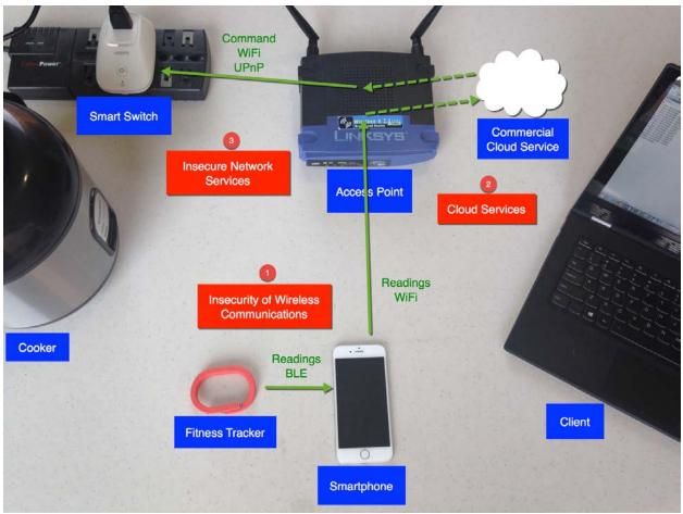
Figure 3: Use case of Powering Devices
