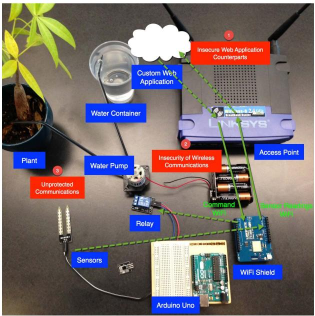
Figure 2: User Case of Remote Watering System
