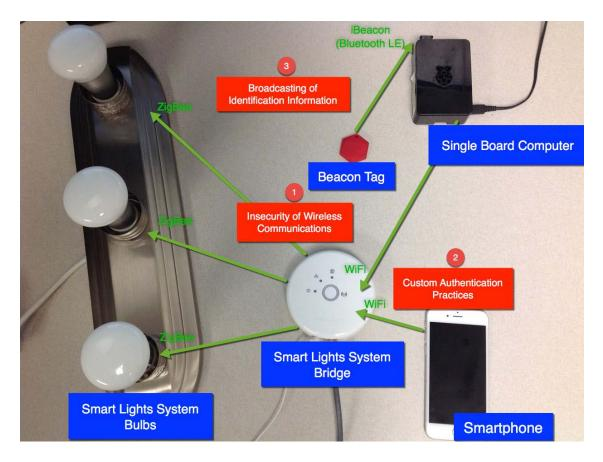
Figure 1: Use Case for Personalized Light Switch System composed of a Beacon tag & a Smart Lights
