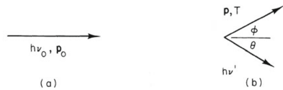
Fig. 15.4 Momentum relationships in Compton scattering. a Before. b After. The photon emerges at angle \theta , the electron at angle \phi
