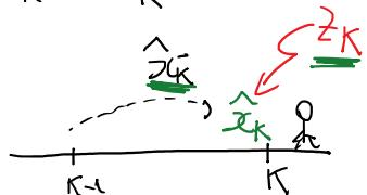
$$\begin{aligned} l_k^- &= x_k - \hat{x}_k^- \rightarrow P_k^- = E[l_k^- l_k^{T-}] \\ l_k &= x_k - \hat{x}_k \rightarrow P_k = E[l_k l_k^T] \end{aligned}$$
