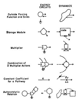
Fig. 10. Comparison of energy circuit symbols with the dynamic symbols of Forrester.
