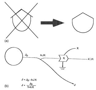
Fig. 11. In the mid 1970s two changes in the language occurred. (a) The storage symbol lost its overhang and (b) a fundamental principle of flow limited source was recognized resulting in a new symbol (the flow limited source).
