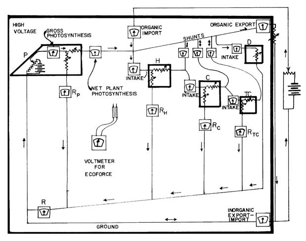
Fig. 2. Analog circuit diagram of the ecosystem energy flow diagram in Fig. 1.
