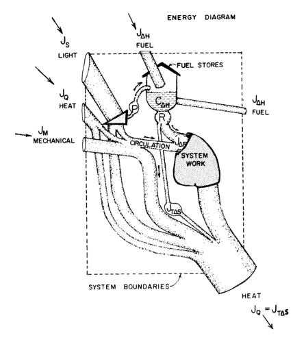
Fig. 5. Energy circuit diagram for an ecosystem showing the main input and output energy fluxes. P, gross primary production; R, total respiration; F, free energy; H, heat of reaction; S, entropy.
