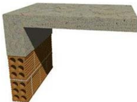
Laje moldada in loco
