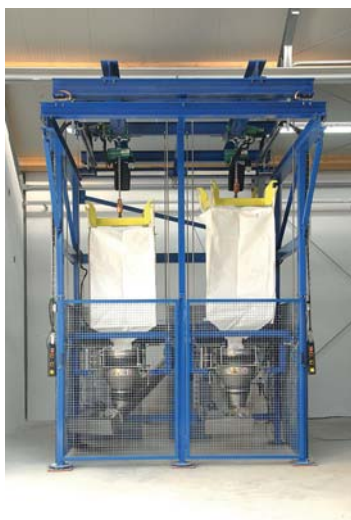
Twin JDN Profi 2 TI hoists, fitted with motorised trolley mountings for big bag handling in chemical, pharmaceutical and food processing environments. (© Hoists)
