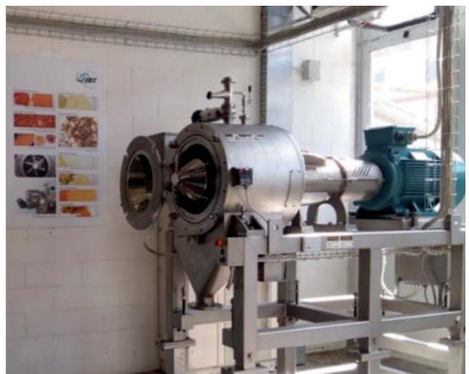
Fig. 2: Cold Extraction Turbo Finisher, FTE-CE at parma pilot plant
