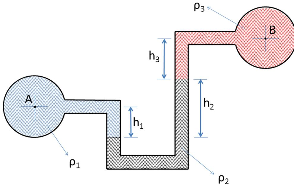
$$P_A - P_B = \gamma_2 h_2 + \gamma_3 h_3 - \gamma_1 h_1$$
