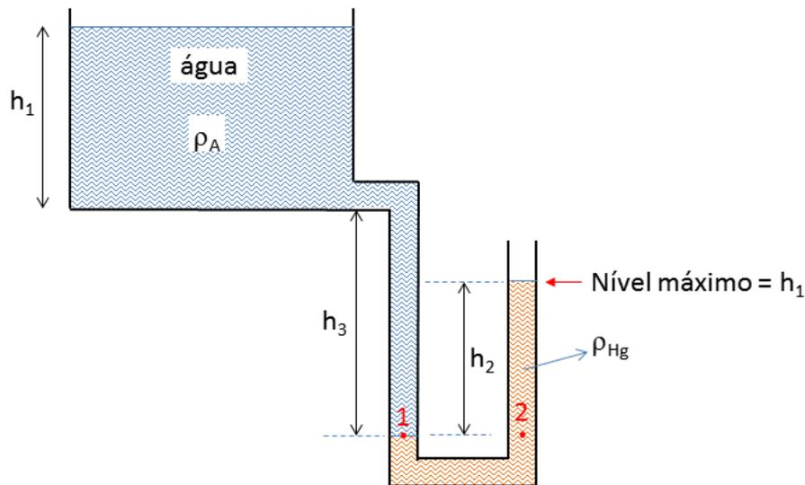
$$\rho_A(h_3 + h_1)g = \rho_{Hg}h_2g \quad \rightarrow \quad h_2 = \rho_A(h_3 + h_1)/\rho_{Hg}$$
