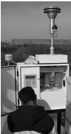
Fig. 2.6. Photo and schematic of sampling device used to measure particles with aerodynamic diameters \leq 2.5\ \mu\text{m} . Each sampler has an inlet (top) that takes in particles \leq 10\ \mu\text{m} . An impactor downstream in the instrument cuts the size fraction to \leq 2.5\ \mu\text{m} , which is collected on Teflon filter. The filter is weighed before and after collection. The Teflon allows construction for other analyses, e.g. X-ray fluorescence to determine inorganic composition of the particles. Quartz filters would be used if any subsequent carbon analyses are needed. Photo and schematic courtesy of US EPA.
