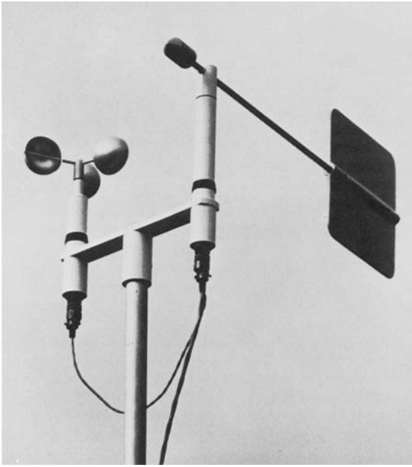
Fig. 21.7. Microvane and three-cup anemometer. Source: Photo courtesy of R. M. Young Co.
