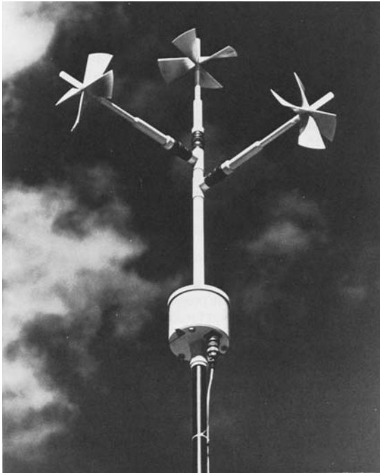
Fig. 21.9. U, V, W wind system. Source: Photo courtesy of R. M. Young Co.
