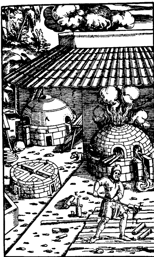
Fig. 1.10. Lead smelting furnace. Source: Agricola, G., De Re Metallica , Book X, p. 481, Basel, Switzerland, 1556. Translated by Hoover, H. C. and Hoover, L. H. Mining Magazine , London, 1912. Reprinted by Dover Publications, New York, 1950.
